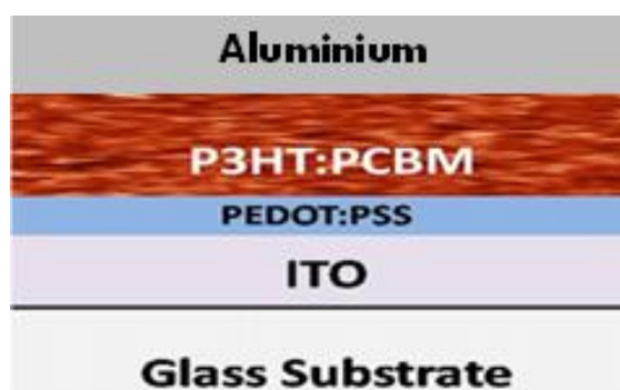
Figure 5.1 Device architecture of reference cell.
