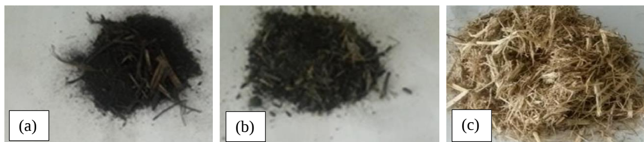
Figure 3-3 As received (a) sugarcane bagasse bottom ash (b) sugarcane bagasse fly ash (c) sugarcane bagasse
