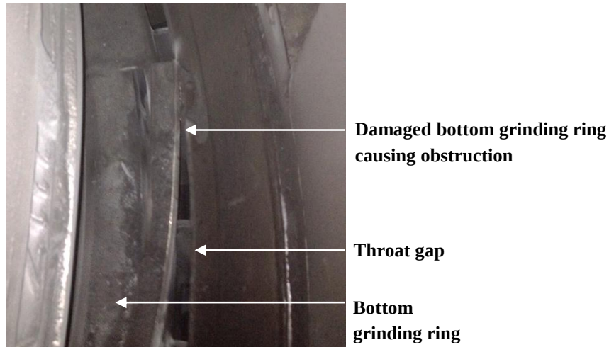
Figure 6.11 Digital image highlighting damaged grinding ring creating an obstruction above the throat gap
