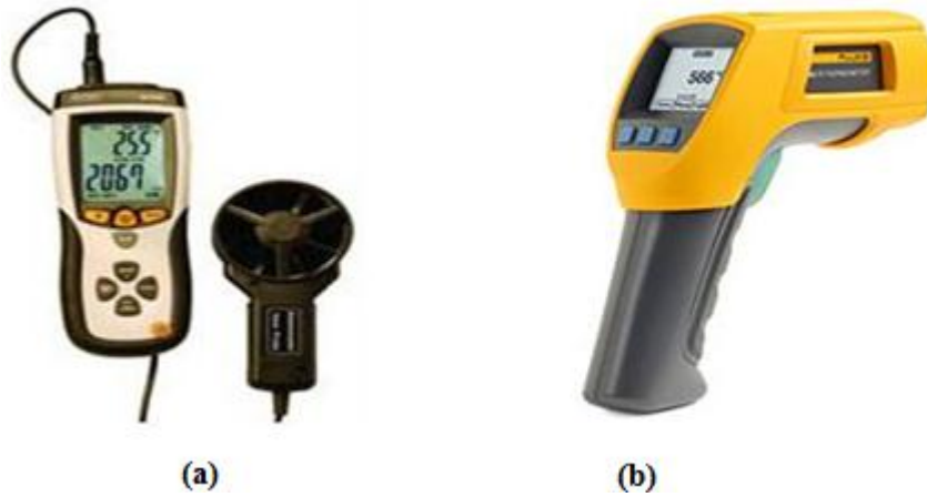
Figure 3.10 Thermo-vane anemometer (a) and infrared thermometer (b) used in the global pulveriser performance tests
