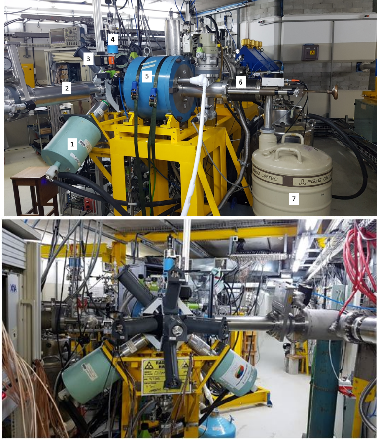
Figure 4.5: Side view of the spectrometer array (upper) showing the 1: LEPS, 2: the beam line, 3: \text{LaBr}_3\text{:Ce} detectors, 4: target ladder, 5: magnetic lens, 6: \text{Si(Li)} cold finger and 7: Dewar used for the measurements. Front view (lower).
