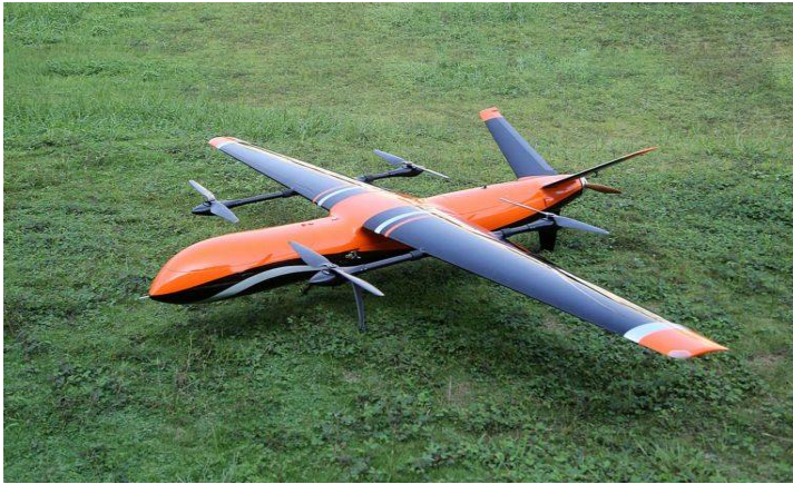
Figure 2.10: Hybrid VTOL RPAS in take-off position (Ridden, 2019)
