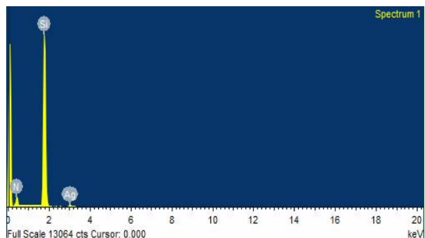
(b) EDS image of Ag NPs deposited for 20 s.
