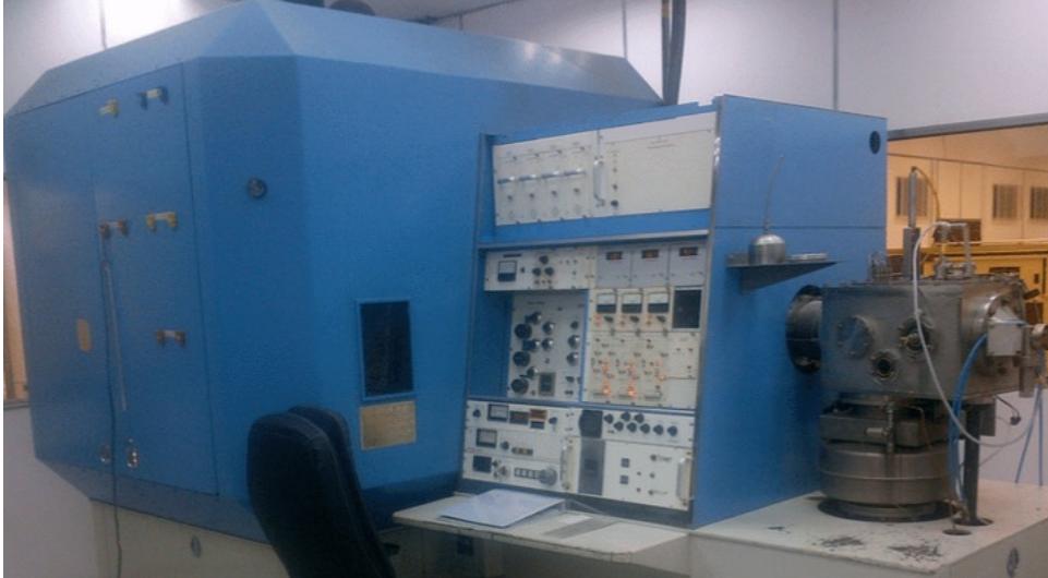
(a) Experimental set-up of the 1.4 MeV Cockcroft-Walton ion implanter.
