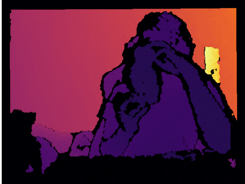
Figure 4.4: Example of colorized output depth retrieved from Kinect V1.
