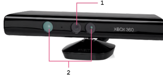
Figure 4.1: Diagram displaying the Kinect V1. Label 1 is the RGB Camera. The components in label 2 work together to become the depth-sensing component. The component on the left is the IR Projector and the component on the right is the IR Camera. Original image by Amos [2011] .
