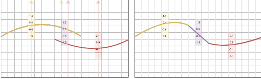
Figure 6.6: Diagram showcasing the method in which information from multiple point clouds is integrated. The diagram on the left shows the average SDF values as a result of the shown rays. The diagram on the right displays the effect of the SDF averaging on the resultant point cloud stored in the voxel block grid.
