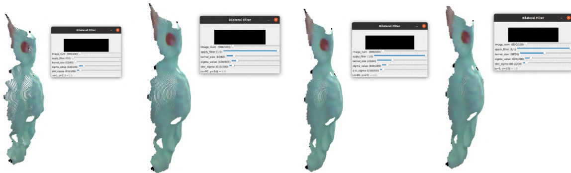
Figure 7.4: Degradation of information showcased through the increasing kernel size in bilateral filtering
