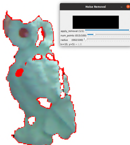
Figure 7.5: Example showcasing the application of the radial outlier removal algorithm. The points highlighted in red are considered outliers and removed when moving to the next step.
