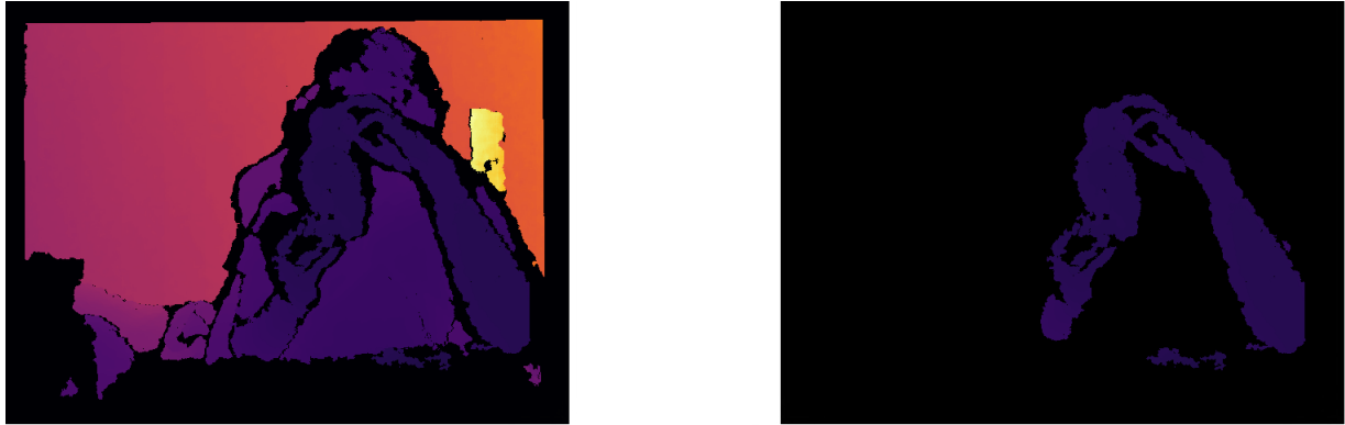
Figure 5.12: Example of depth thresholding image. Range selection for viable depth values is calculated from depth at hand landmarks.
