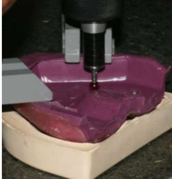
Fig 10. Point probe CAD scanner scanning an impression coping in the PVS impression in its special tray. All impression trays were placed on a flat custom-made base to prevent movement during scanning.
