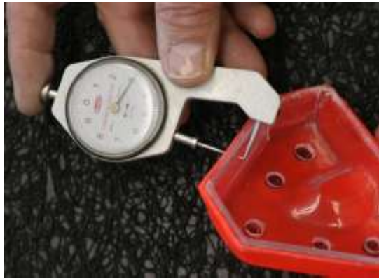
Fig 2. Vacuum-formed 3mm spacer
