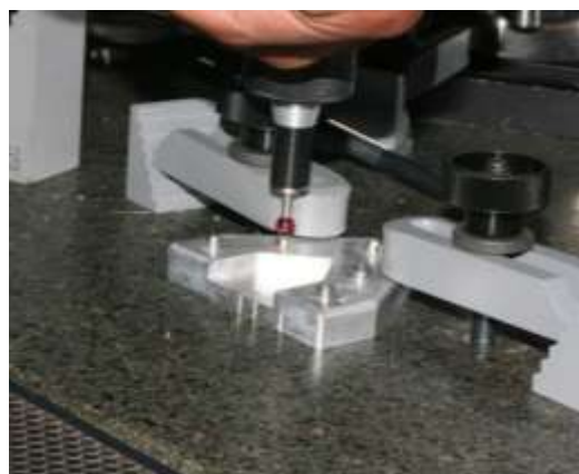
Fig 9. Point probe laser scanner on master model.
