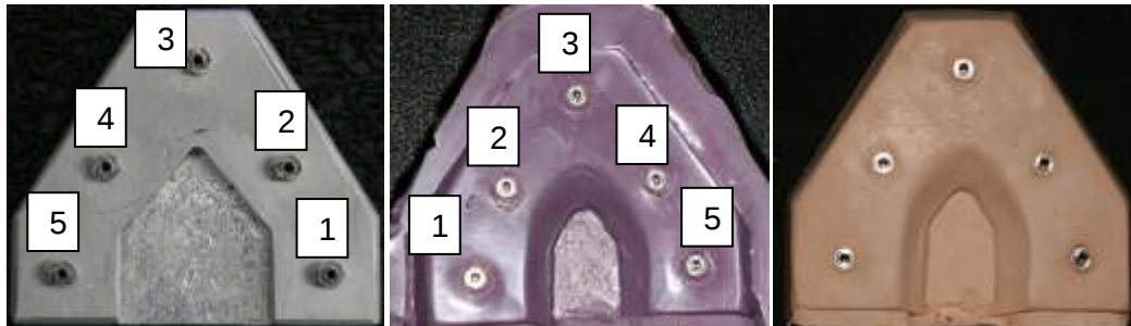
Fig 8. Measurements taken on the master model, the impression and the master cast for the 5 implant positions numbered 1-5: each inter-implant distance was measured.
