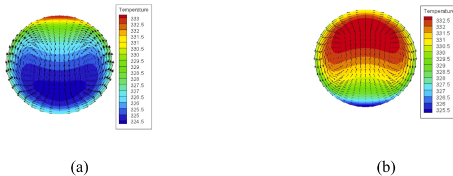
Fig. 4. Cross-sectional view of temperature contour and velocity vector (a) at heater (b) at cooler [37]. Copyright © 2015 Elsevier Masson SAS.
