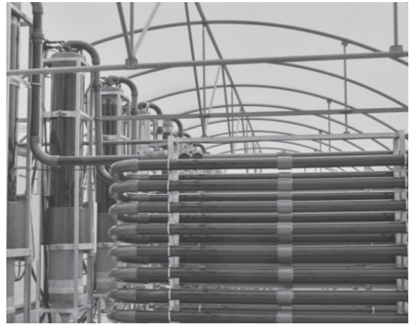
Horizontal tubular system
