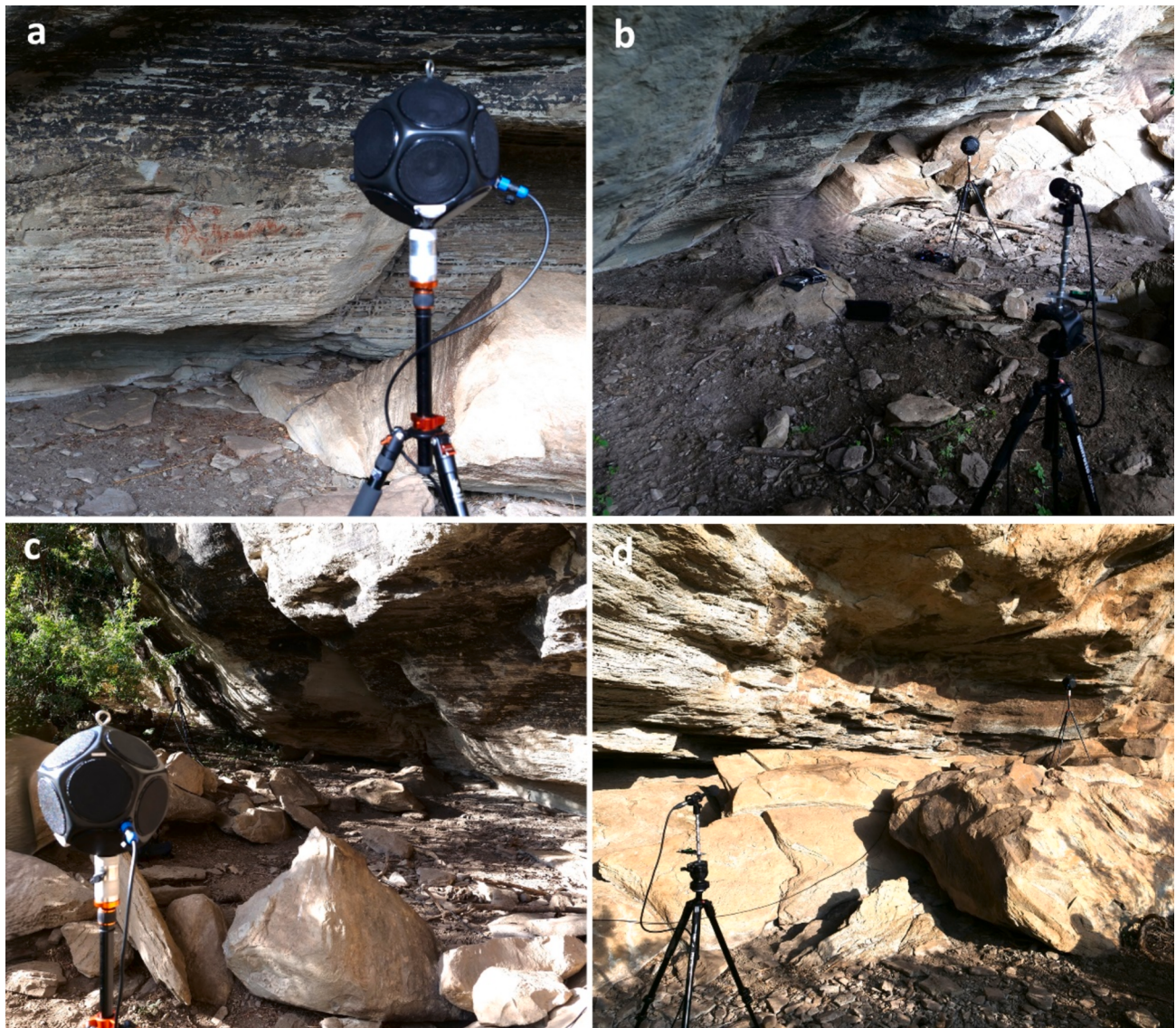
Fig. 4. Example of sound source positions used in Barnes I set according to the established criteria: (a) detail view of S1 in front of a dance scene; (b) General view of S1 and the receiver in R1; (c) General view of S2, placed in front of S1 at a central location, and the receiver in R1; and (d) S3 on the top of rocks to cover the right part of the shelter, with the receiver in R3.
