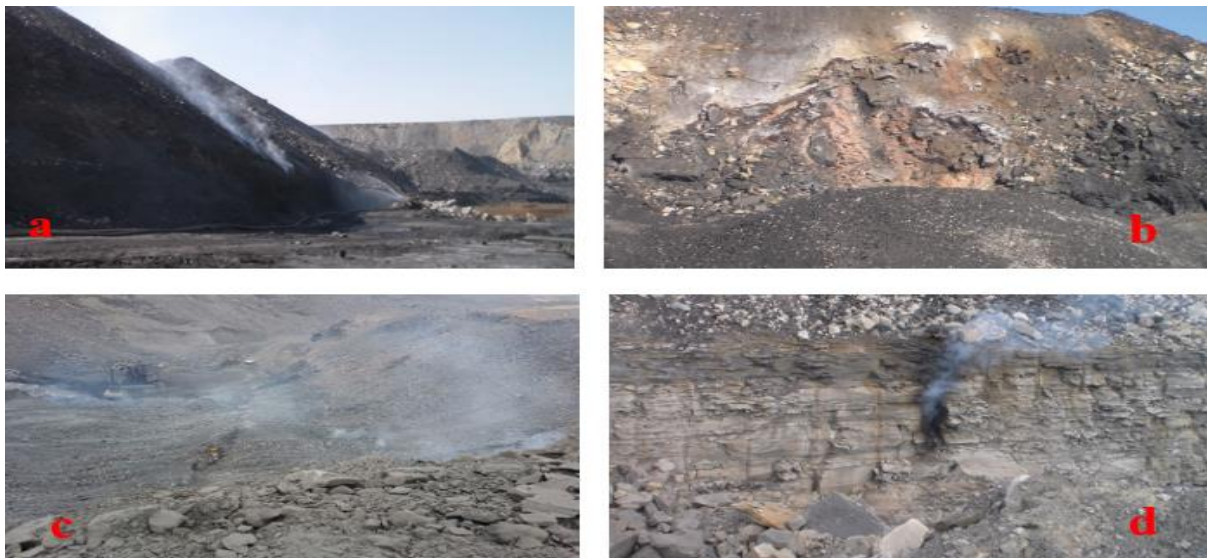
Figure 1.2 (a) Self-heating of run-of-mine and (b) spoil heaps at Tweefontein Mine (c) Signs of self-heating in coal seams at Khwezela Mine (Bokgoni Pit) and (d) self-heating of in-seam shale at Goedgevonden Colliery, Witbank, South Africa
