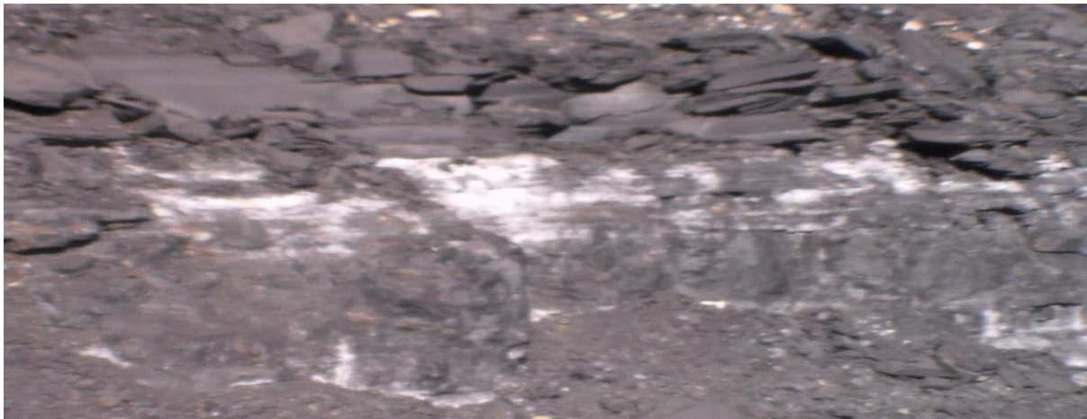
Figure 4.9 Forms of crystals and ammonium chloride present on the surface of coal-shale at iMpunzi Mine, Witbank, South Africa
