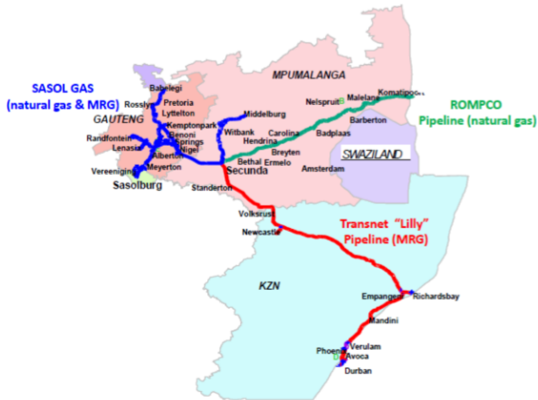
Figure 5.2: Main gas transmission and distribution lines on South Africa (Price Waterhouse Coopers, 2015)
