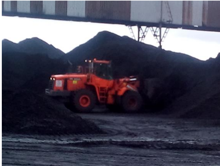
Figure 6: Front end loader stock piling at coal stock yard
