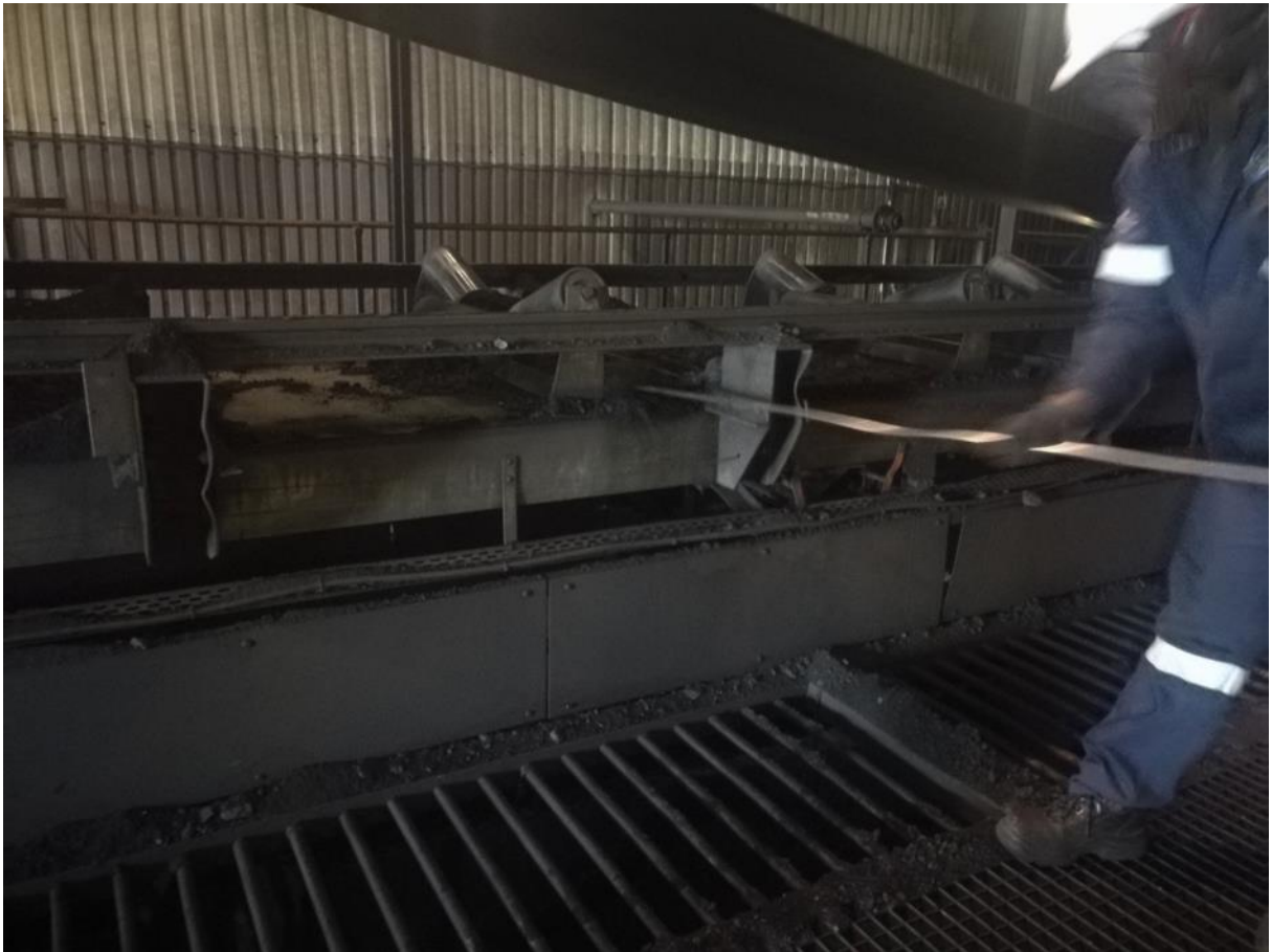
Figure 9: Cleaner sweeping coal underneath a conveyer belt
