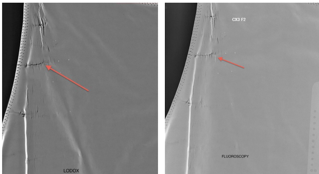
Figure 8: Example of an imaged lead apron imaged with Lodox Stascan (image cropped to demonstrate only the relevant part) and Fluoroscopy, depicting corresponding lead apron fractures (arrows).
