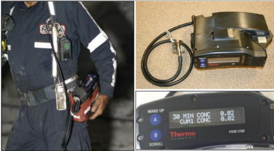
Figure 3.4 Real-time Continuous Personal Dust Monitor (CPDM)/PDM3700 (National Academies of Sciences, Engineering, and Medicine, 2018; Belle, 2017)
