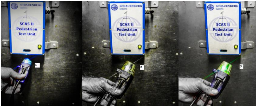
Figure 5.38 Virocap PDS Test: Blue Flashing LED (1); Yellow Flashing LED (2); Green Flashing LED
