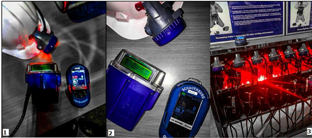
Figure 5.13 Methane gas alarm (1), ‘Methane (Ch4) Evacuate’ message on PTC Lamp (2), Nearby PTC Camp alarming (3)
