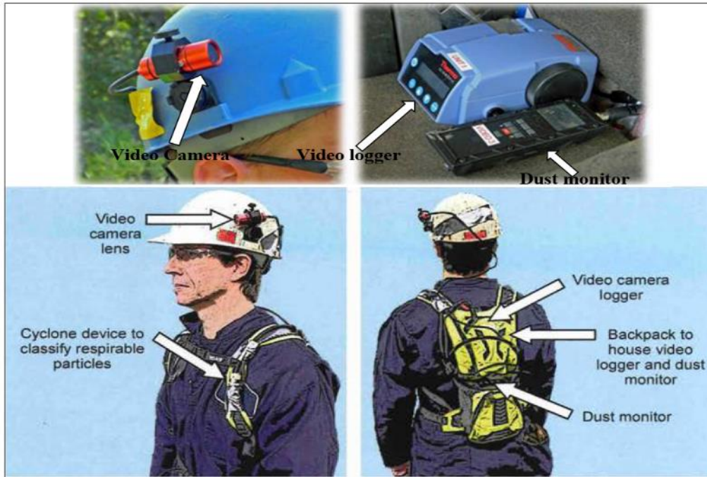
Figure 3.5 Typical Helmet-CAM technology Setup on a miner (Cecala & O'Brien, 2014; Haas, et al., 2016)
