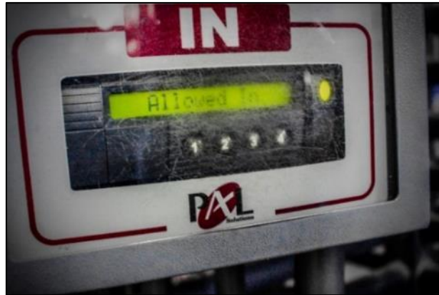
Figure 5.39 T &A Swipe Access Point Message after miner complied with all Gate Rules
