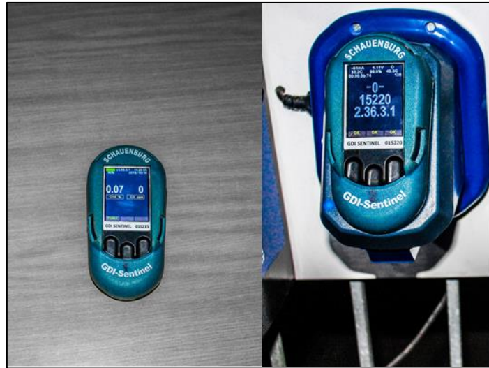
Figure 5.10 Sentinel Handheld GDI (1) on a table, (2) charging
