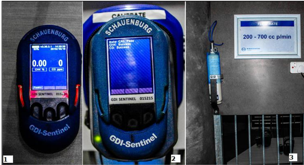
Figure 5.12 showing an uncalibrated GDI (1); calibrated (2) GDI; calibration gas canister (3)
