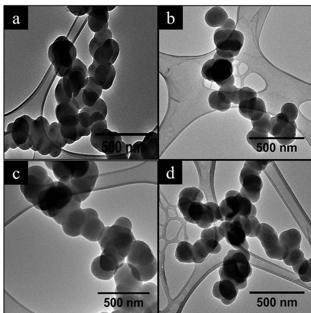
Fig. 1 TEM images of carbon spheres obtained using two different carrier gases; (a) CSs-H<sub>2</sub>; (b) NCSs-H<sub>2</sub>; (c) CSs-Ar and (d) NCSs-Ar, respectively.
