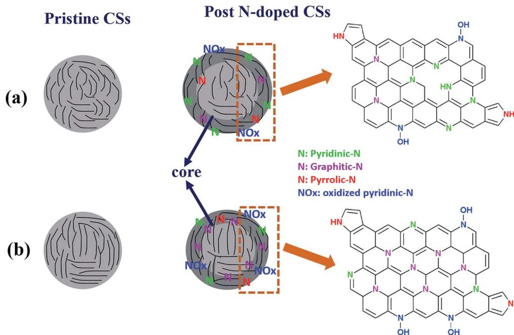
Fig. 6 Possible mechanism showing the role of carrier gas on the N-configuration of the CSs synthesized in the presence of (a)  $H_2$  and (b) Ar, respectively.
