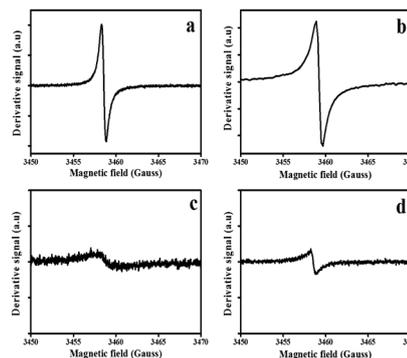
Fig. 5 Electron spin resonance spectra of the pristine and N-doped CSs; (a) CSs-H<sub>2</sub>, (b) NCSs-H<sub>2</sub>, (c) NCSs-Ar and (d) NCSs-Ar, respectively.
