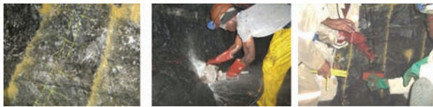
Figure 7—(a) Marked off sample section, (b) cutting sample from stope face, and (c) chipping samples from stope face (source: Hol, 2009)
