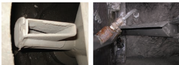
Figure 5—(a) Vezin sampler splits the primary residue sample, and (b) cleaning nozzle pointing at head grade sampling by cross-stream cutter (source: Kelly, 2007)
