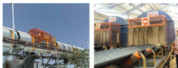
Figure 3—Go-belt sampler installation on conveyor belts from shaft head (source: Letsie, 2009; Minnitt, 2013)
