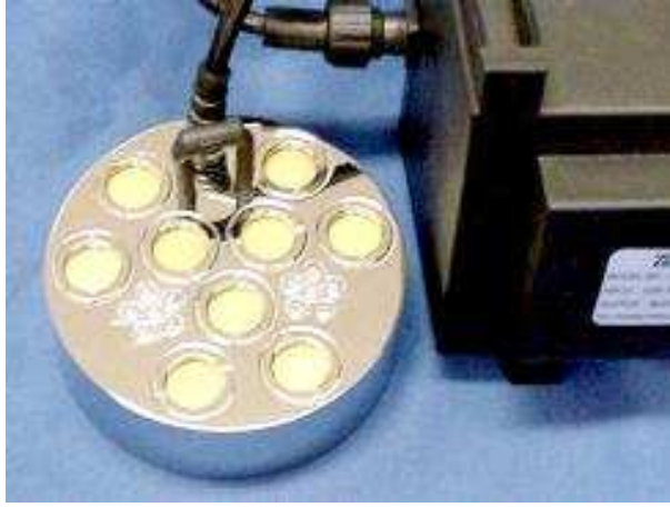
Figure 3.2: A photograph of the ultrasonic transducer that was used to produce droplets through out the present study
