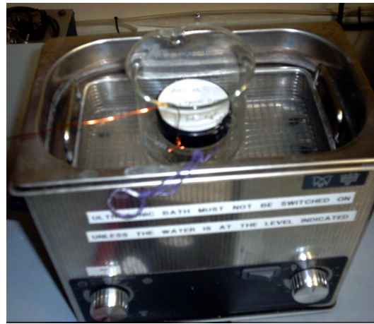
Figure 3.3: A photograph showing (a) the work table with starting materials and other allied equipment (b) the ultrasonic bath where substrate could be cleaned before deposition
