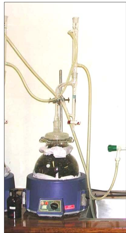
Figure 2.5. A clewenger apparatus used in hydrodistillation of essential oils.
