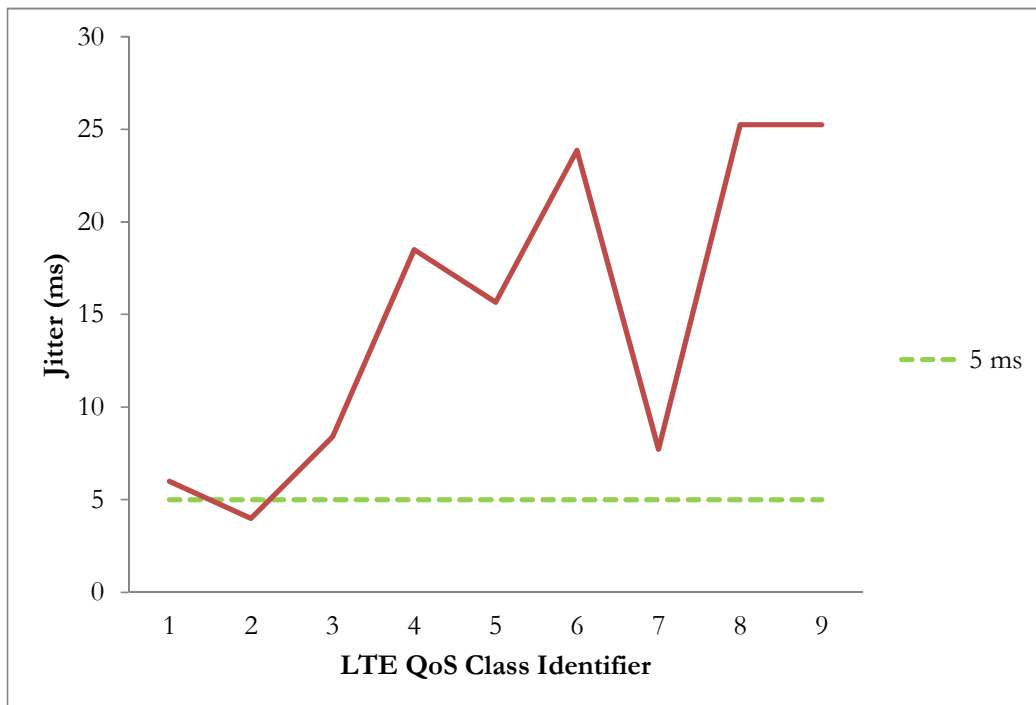
Figure 6-3. Jitter on Differing LTE QoS Class Identifier (QCI) Types
