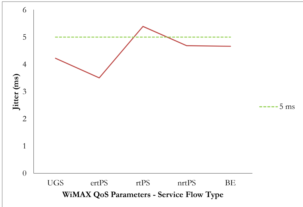
Figure 6-6. Jitter on Differing WiMAX Service Flow Types [11]
