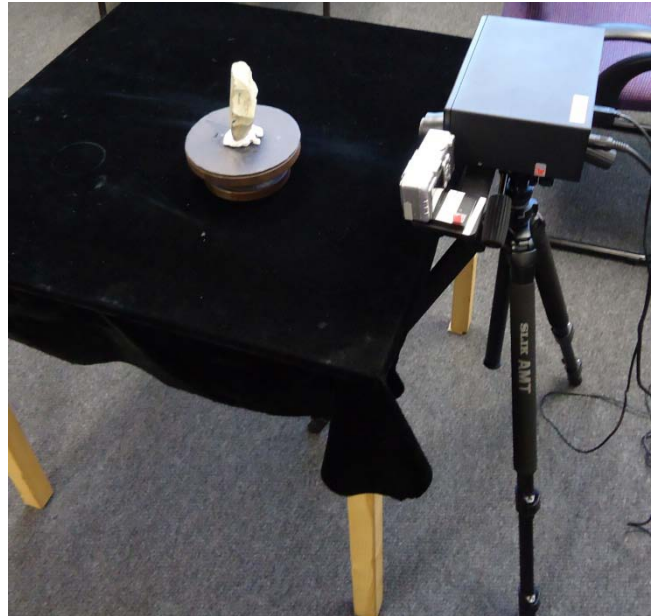
Figure 3: Depicting Real Scan USB scanner, table and scanning stand
