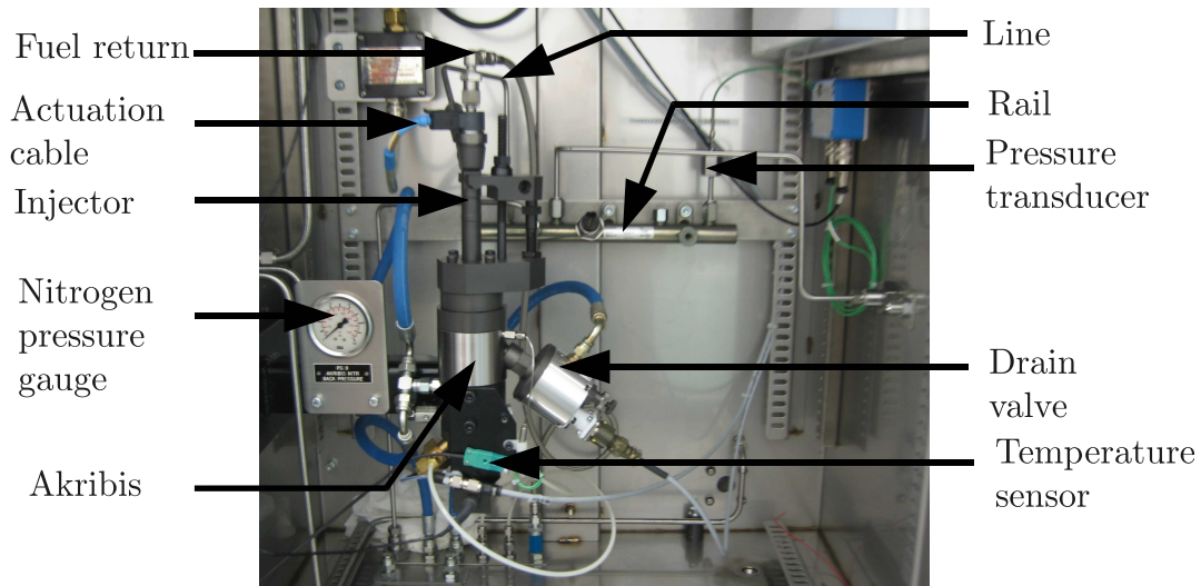
Figure 7.1: Photograph showing the injector, rail, Akribis and fuel lines for the test stand.
