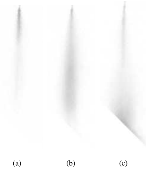
Figure 3.3: Images at 10 MPa opening pressure for a three orifice injector with diesel fuel.
