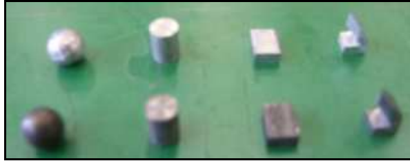
Figure 7: Aluminium and steel particles used for the experiments
