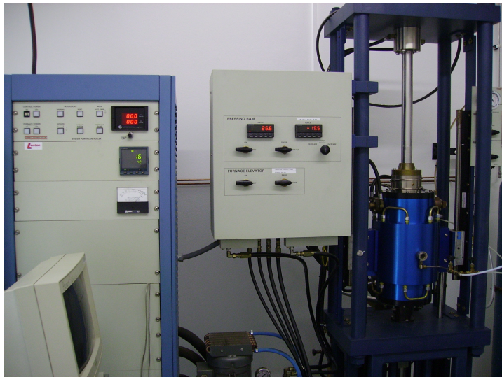
Fig3.7: The Uniaxial Hot Press used for sintering
