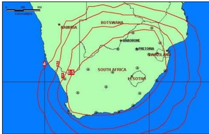
Figure 3.3: Projected location accuracy (km) of cloud-to-ground lightning flash data for the SAWS LDN from the VAISALA NPEP model (VAISALA)
