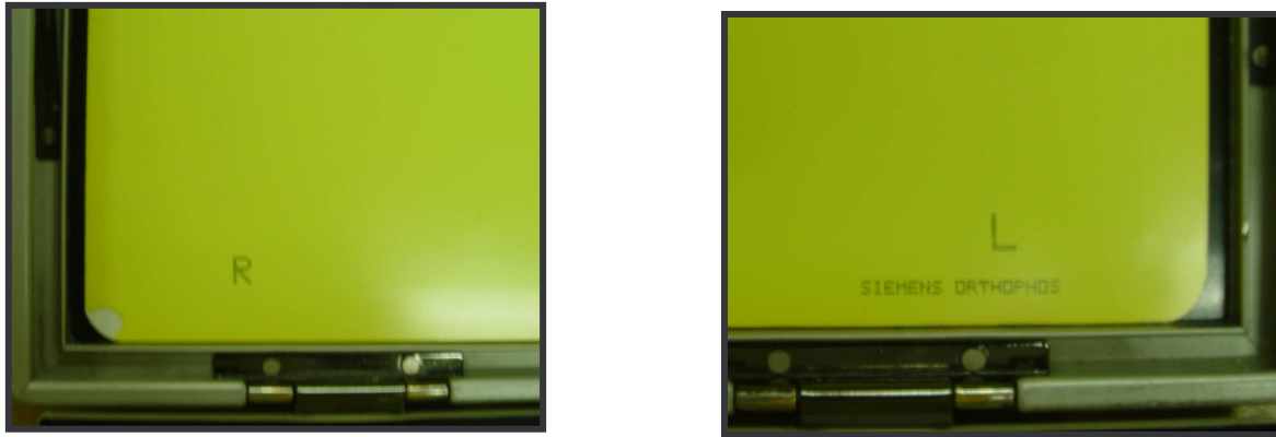
Figure 3.8 – ‘R’ and ‘L’ digital markers on panorex cassette
