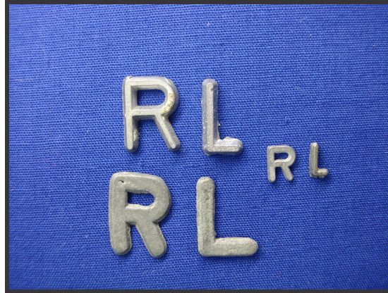
Figure 3.10- Variety of lead markers: 'R' and 'L'
