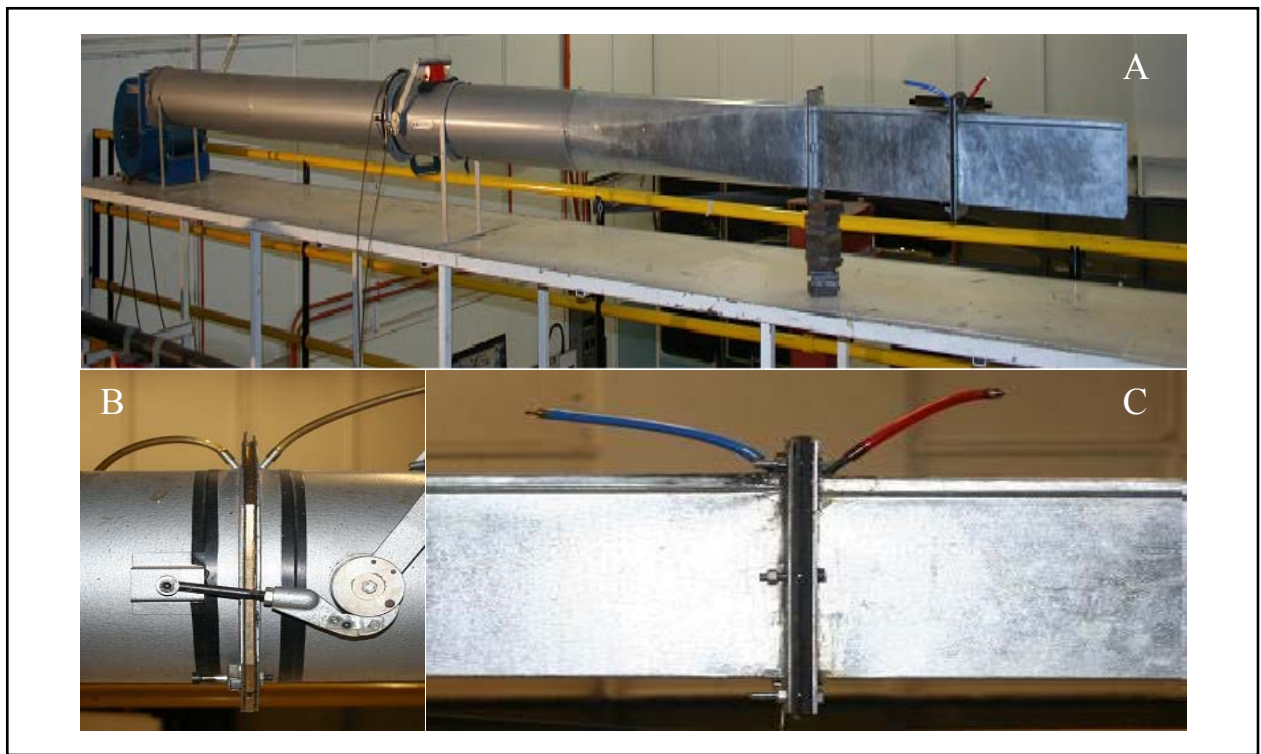
Figure 20: Photographs of the Calibration Duct
