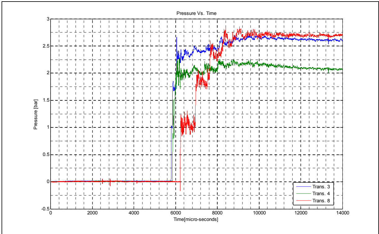
Figure 40: Unfiltered Pressure Traces for P11Fr&P13Fr - M_{set} = 1.42 , P_o = 0.83 bar
