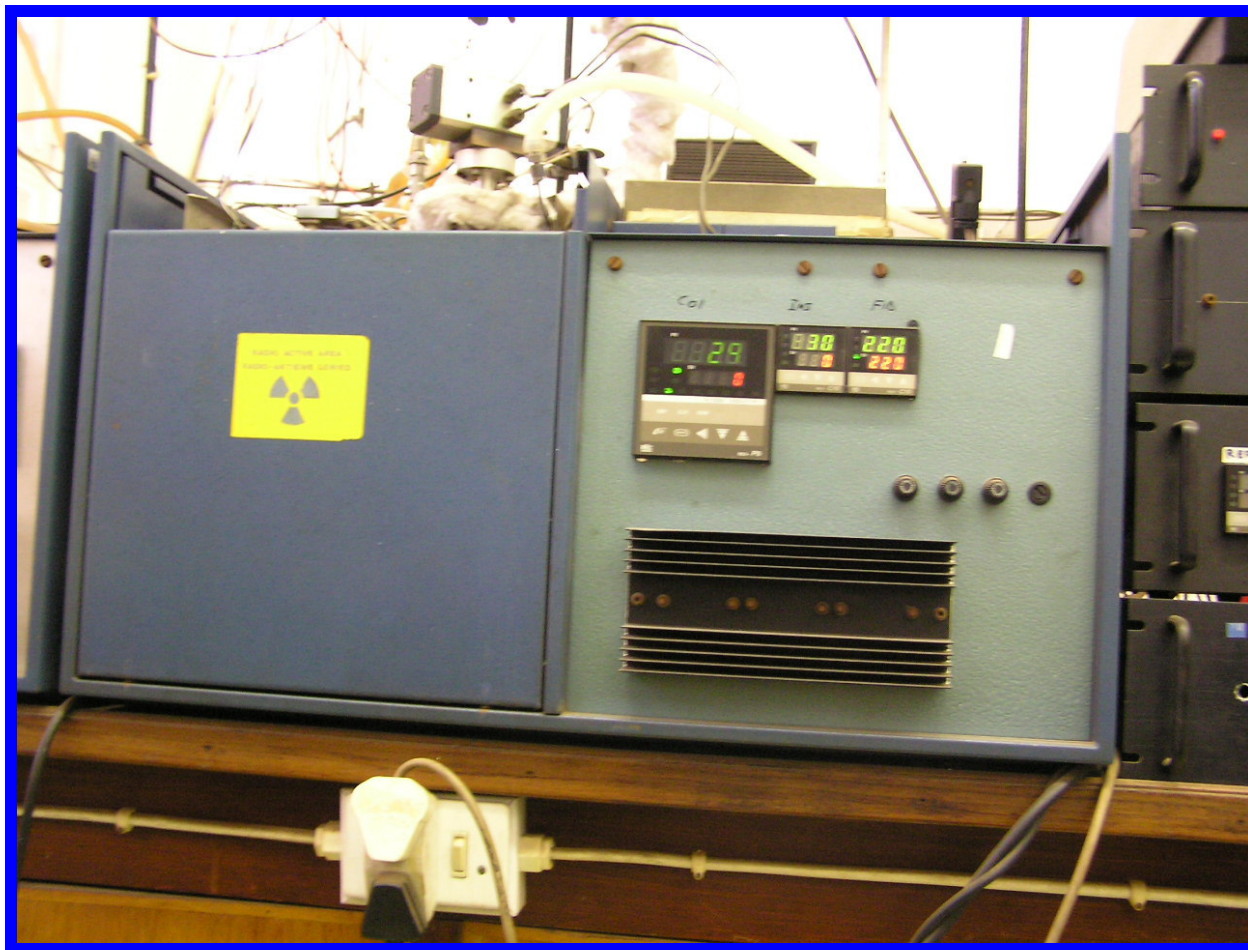
Figure 3.3: A picture of an off-line GC apparatus equipped with a capillary column and used to separate reaction products.
