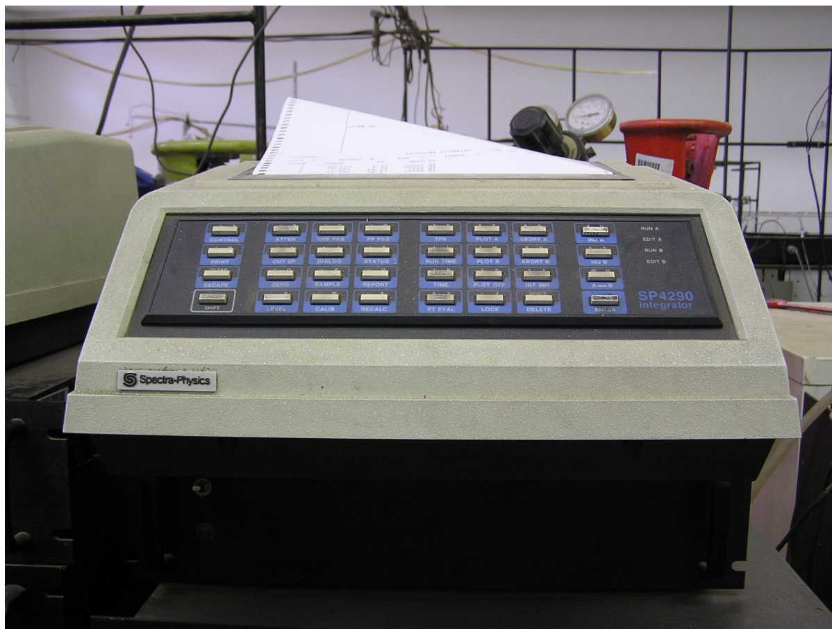
Figure 3.4: A picture of an integrator apparatus used for GC output.
