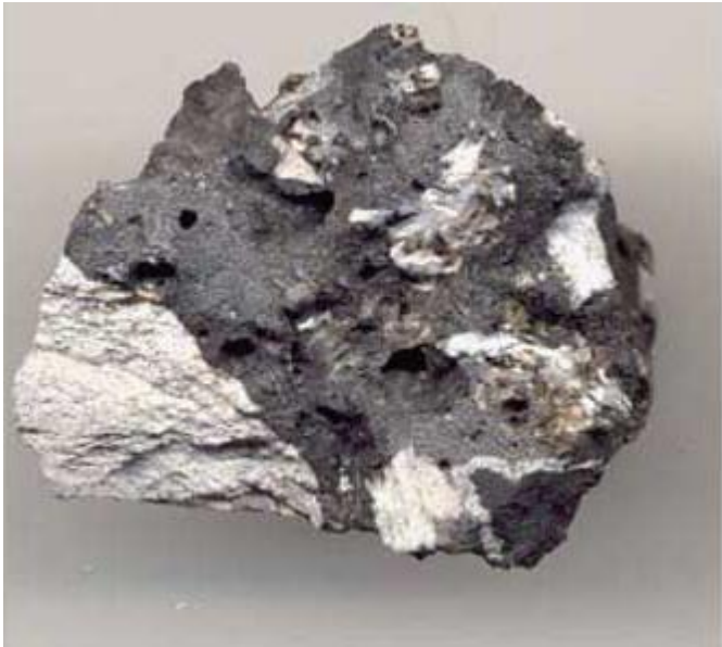
Figure 3.3: An image of a hand-picked sized sample of a coarse gasification ash/clinker similar to the one used 12
