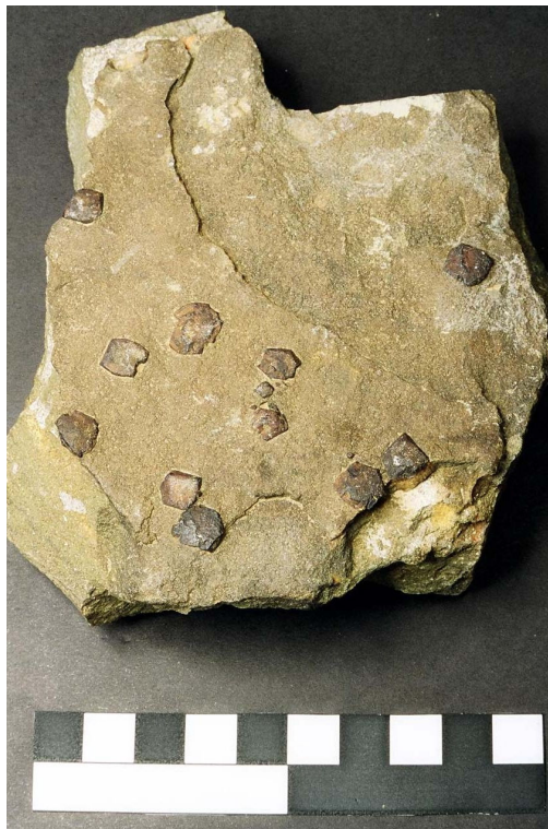
Figure 30: Pyrite crystals within a massive sandstone, Bucklands. (Scale: 10cm scale bar).
