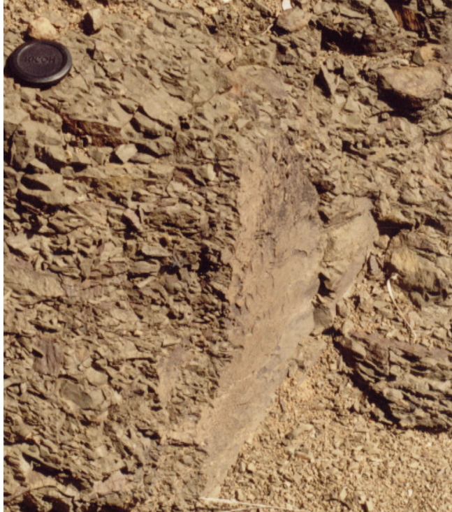
Figure 25: Slickensided surface within the overbank depositional environment, Bucklands. (Scale: 6 cm lens cap).
