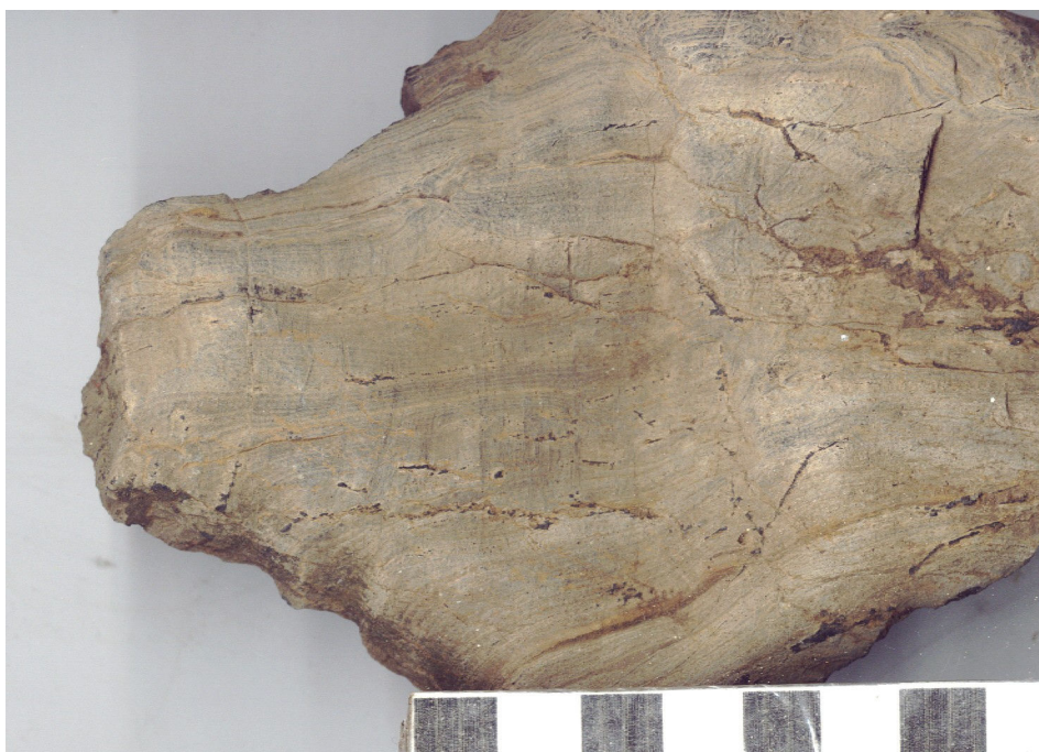
Figure 28: A sample of limestone, displaying wavy lamina, from The Grant (1cm minor divisions on scale bar).
