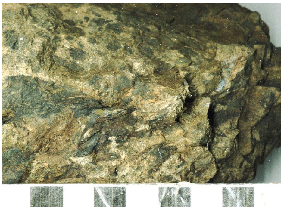
Figure 36: Intraformational conglomerate comprising sub-rounded mud clasts in a sandstone matrix. (1cm divisions on scale bar).
