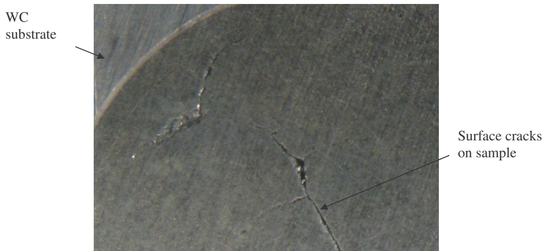
Figure 4.19: SEM micrograph of sample 1 sintered at 5.5GPa and 900 0 C using a high pressure apparatus showing surface cracks.
