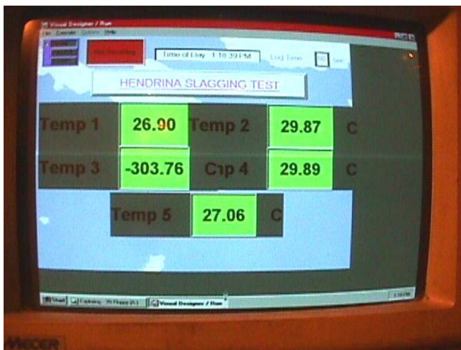
Figure C.7: Computer screen showing the temperatures at the start of a run. The high negative temperature is indicative of a faulty thermocouple.
