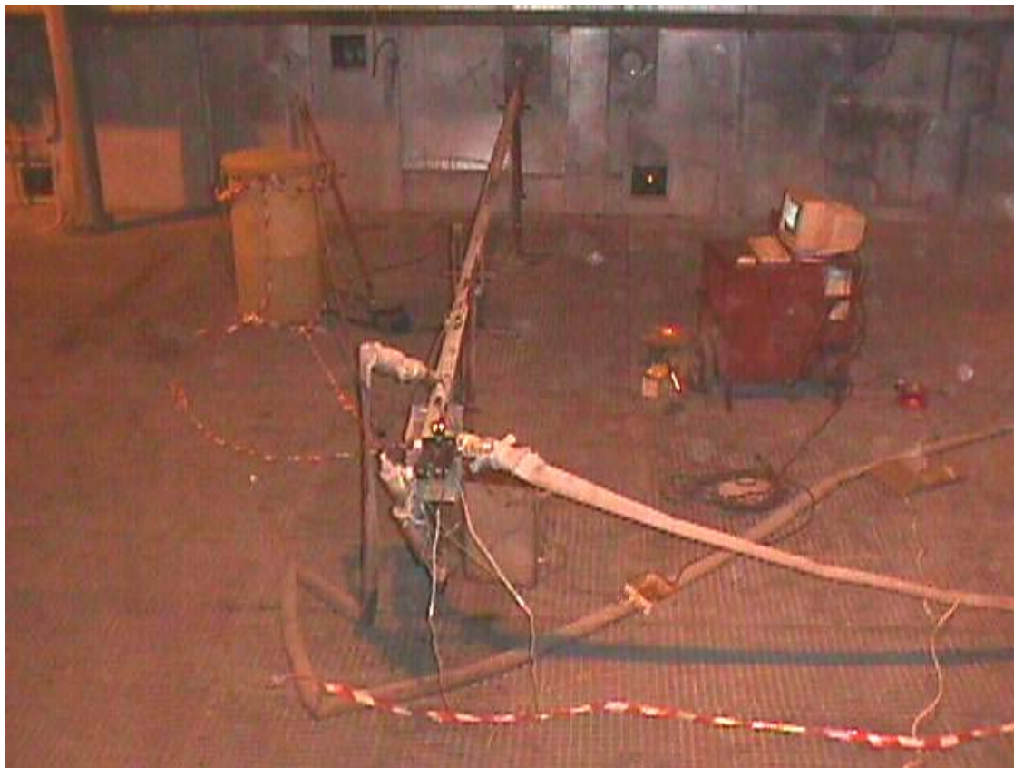
Figure C.3. Suction pyrometer at hole 4.
