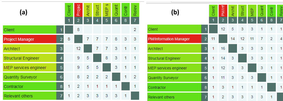
Figure 7.19: People-People interaction DSM (weighted (showing edge values) (a) pre-B (b) BIM-enabled Team member node colours denote their criticality ranging from Red (highest) to Green (least)
