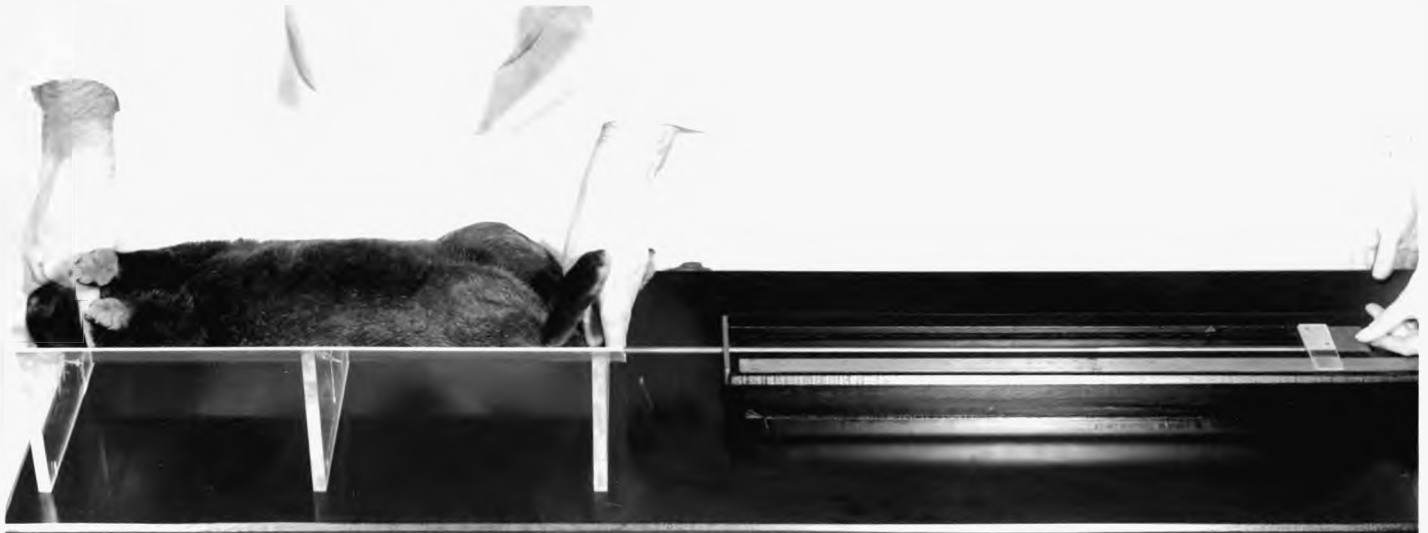
Figure 1. The measuring board used for body length on anaesthetized rabbits. A black rabbit is shown for photographic clarity.
