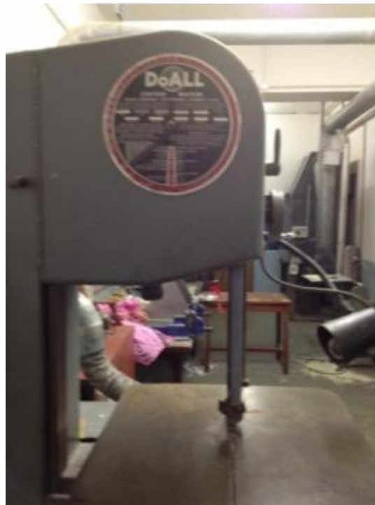
Figure 3.4: Image of the DoALL band saw which was used to cut composite plates
