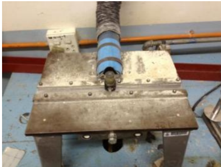
Figure 3.6: TensilKut diamond shaping tool used to shape the tensile dog-bone specimens
