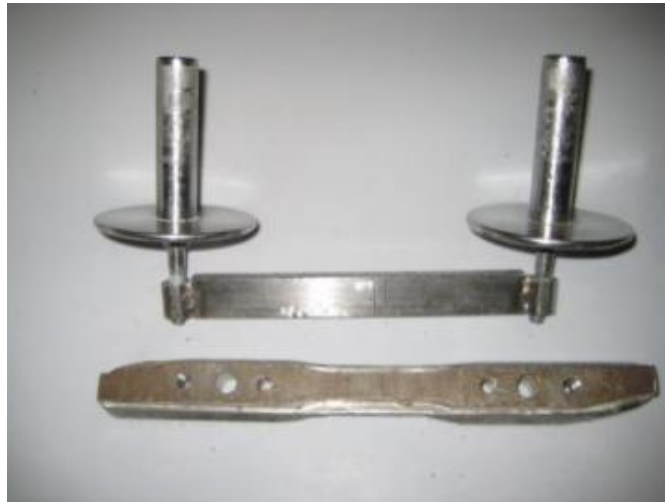
Figure 3.5: Stainless steel template used to hold the rectangular tensile specimen during shaping
