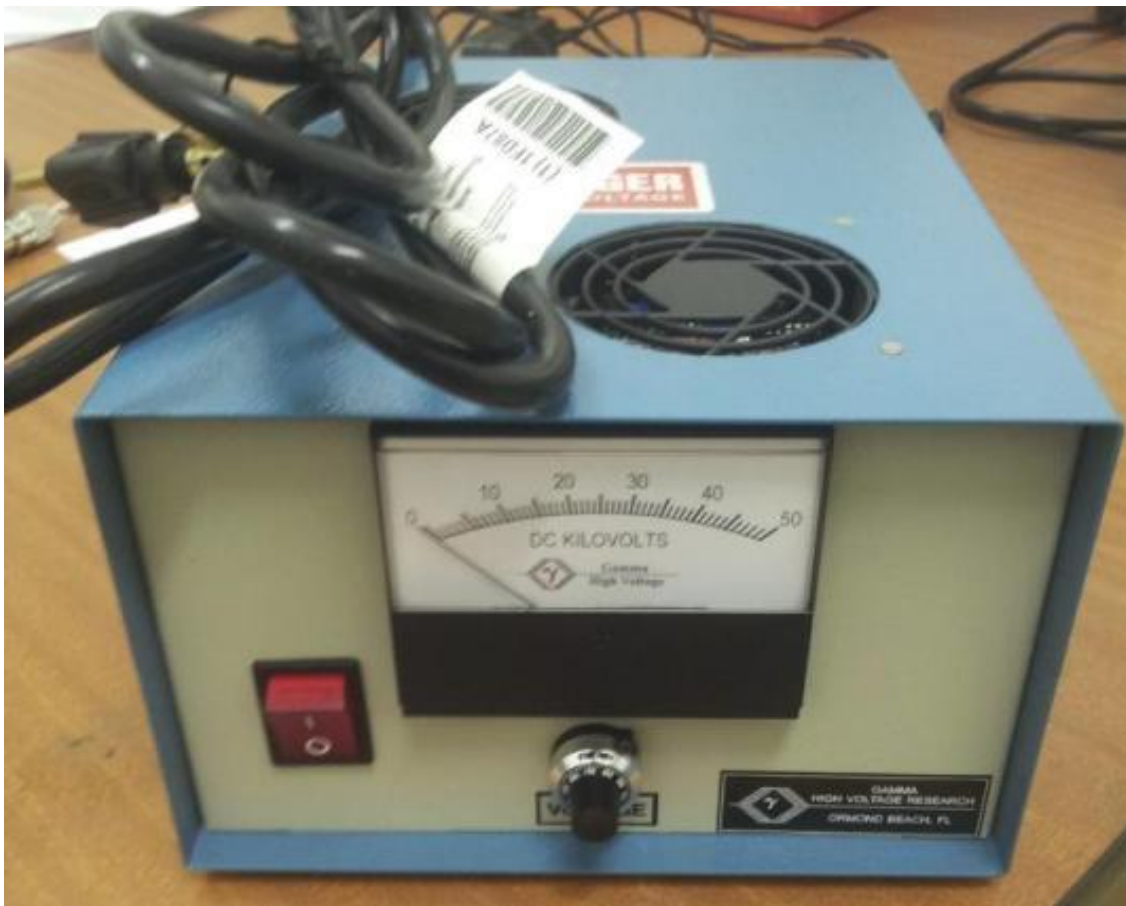
Figure 3.10: High voltage power supply used to supply the electric field for the electrospinning process
