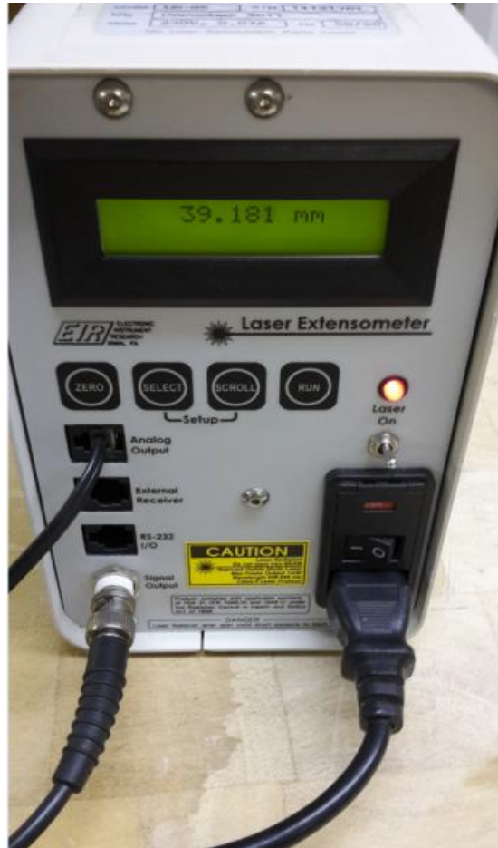
Figure 3.20: Laser extensometer used to measure the jaw displacement under tensile loading
