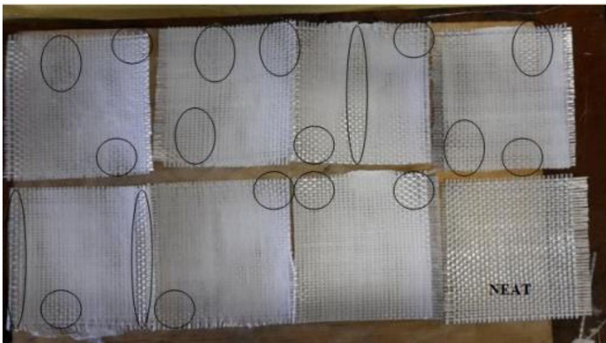
Figure 4.9: Image showing poor dispersion of PAN nanofibers collected on the woven glass fiber mats
