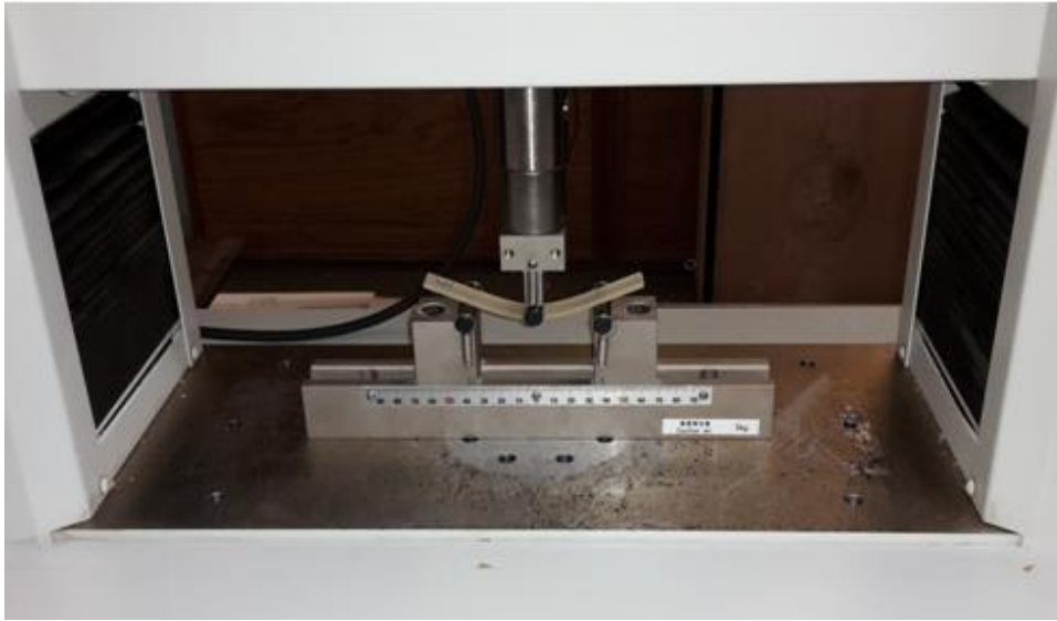
Figure 3.22: Close up image of the 3-point flexural test attachment during a test
