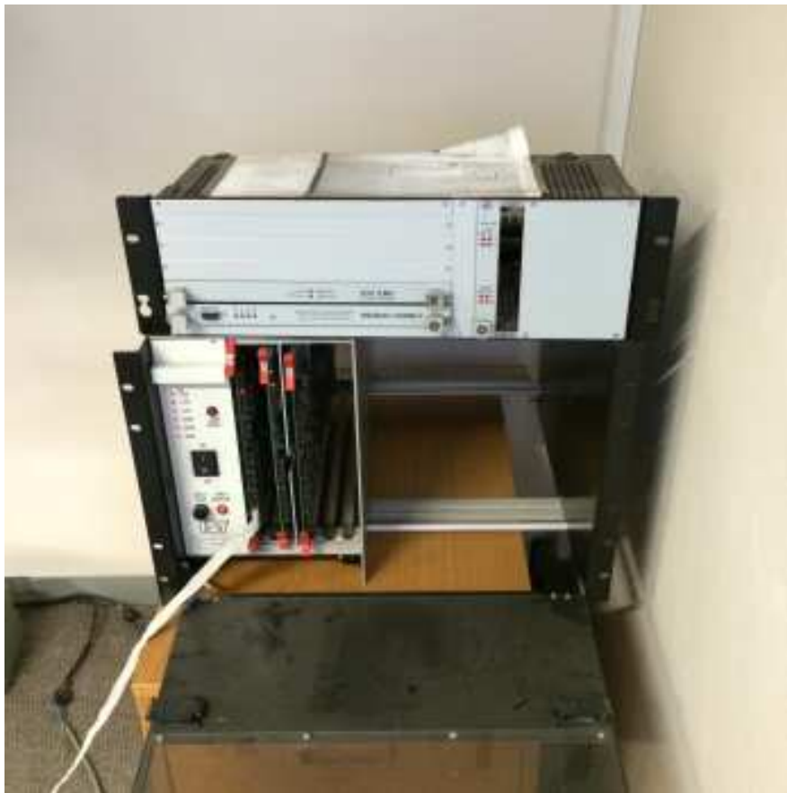
Figure 7.2 Illustration of a D20 RTU and the IST ERTU used for the simulation and experiment
