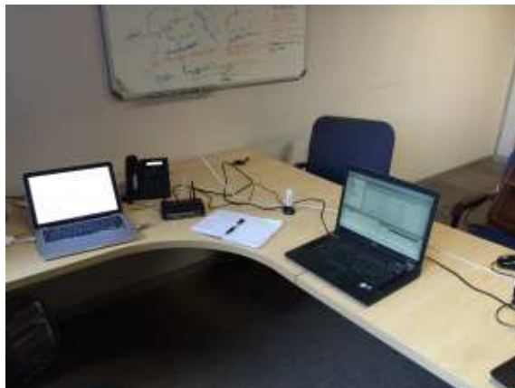
Figure 7.5 An illustration of the switch and the MacBook Laptop connected to generate traffic and to try and send messages to the network
