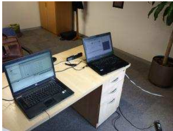
Figure 7.4 The HP laptop running the SCADA simulator and RS232-TCP/IP conversion which transmits the data to the Toshiba laptop's GNS3 network via a network switch
