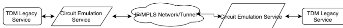
Figure 4.3 An illustration of the circuit emulation implemented in MPLS for legacy services (Alcatel-Lucent, 2011)
