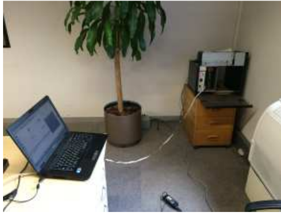
Figure 7.3 The Toshiba laptop running the MPLS/IP core network on GNS3 simulator, TCP/IP-RS232 conversion and it is connected to the RTU via RS232
