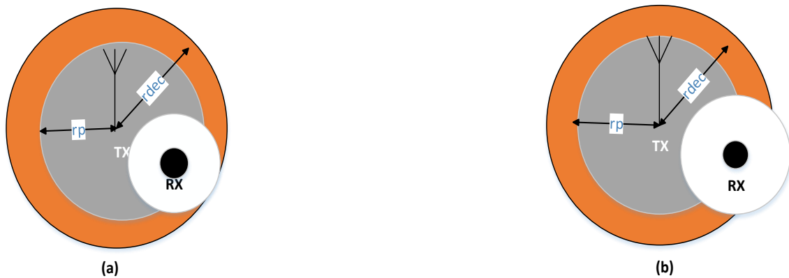
Figure 2.8 Primary transmitters protection area and receivers decoding area for low and high transmit powers. [28]
