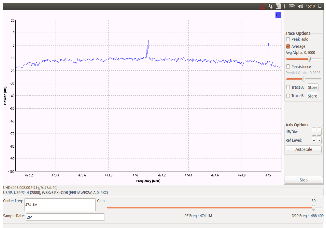
Figure 4.12 Spectrum analyser showing the FFT magnitude of channel 21.
