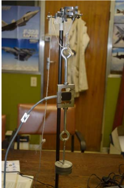
Figure E.1: Setup used in the calibration of the hinge moment loadcell through the application of load directly to the loadcell.
