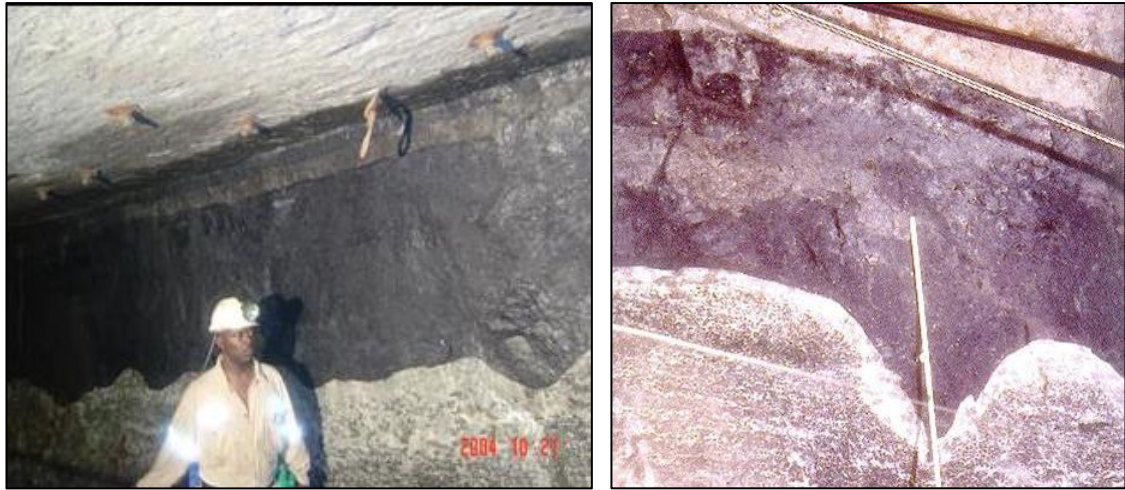
Figure 3-4 Examples of footwall variability in Lonmin's UG2 operations, explaining high relative short range variability component observed in UG2 Reef thickness. (Photos courtesy of Lonmin)
