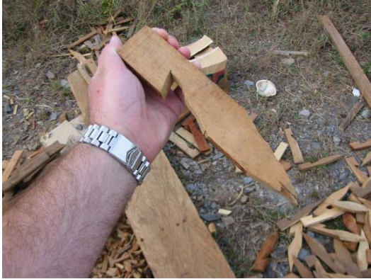
On-site manufacture of wooden pegs.
