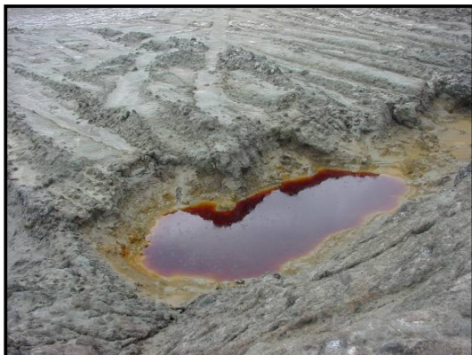
Figure 2.2.7: ARD at the toe of a tailings facility
