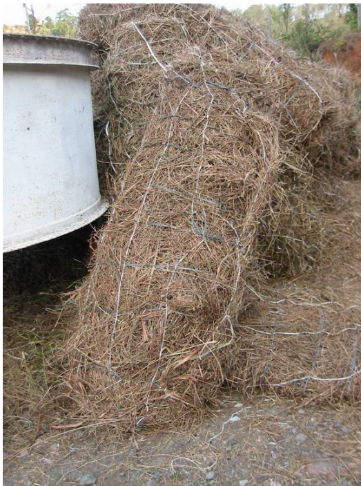
Rolls of grass mats. Fertiliser and seed are included in the grass matrix.
