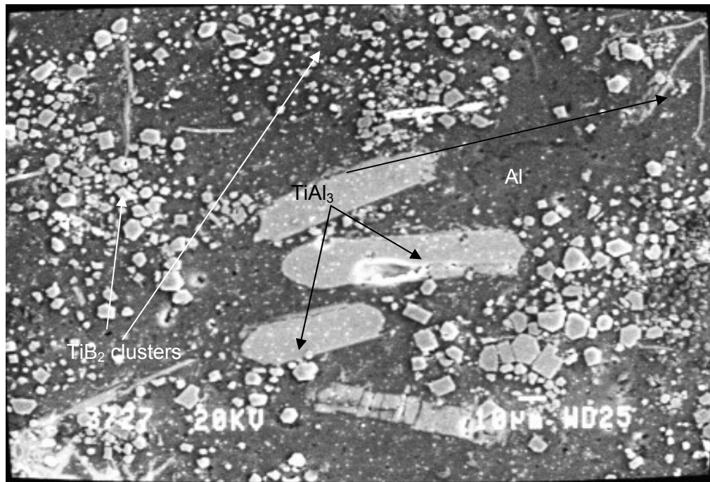
Figure 4 6: Large TiAl 3 particles and TiB 2 particles in alloy Ind1B
