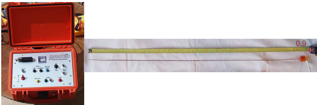
Figure 6: MREL Microtrap & VoD proberod
