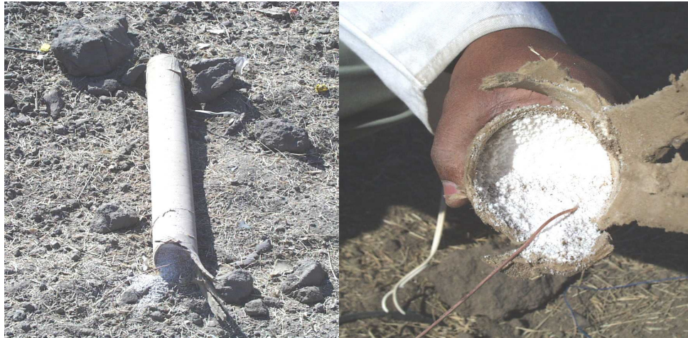
Figure 13: Undetonated explosives below critical diameter
