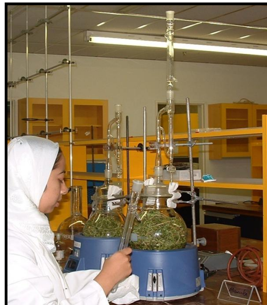
Figure 2.3 Clevenger apparatus being set up.
