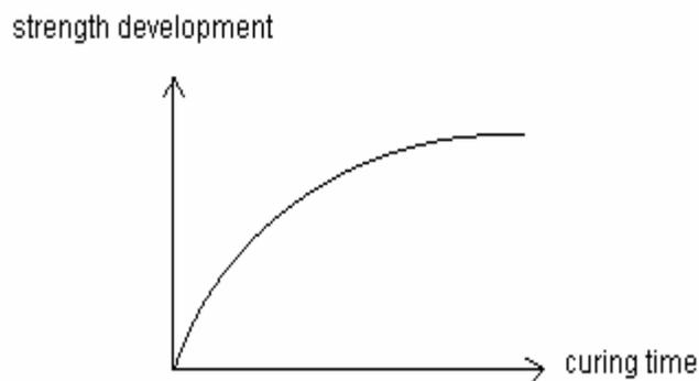
Figure 5.1 Illustration of strength development in cement stabilised materials
