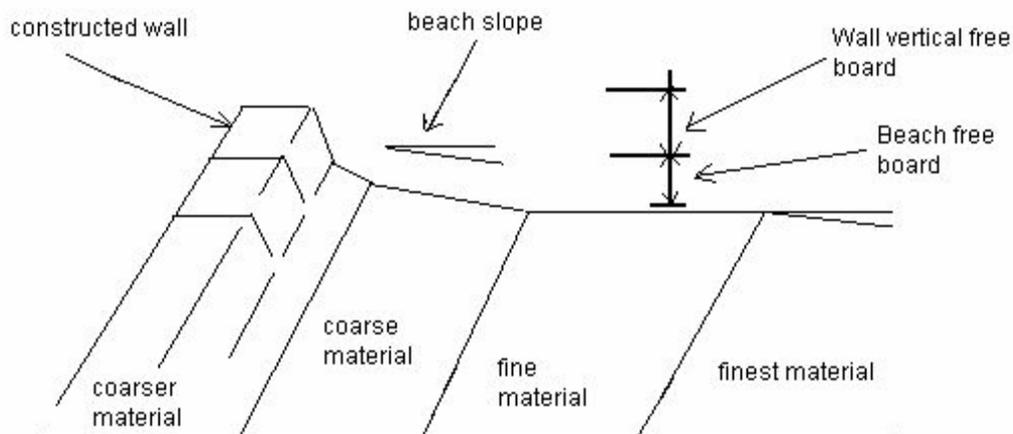
Figure 3.7 Principles of Spigot Deposition (Chamber of Mines, 1996)
