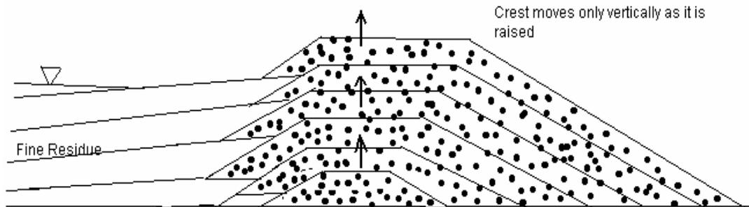
Figure 3.5 Centreline tailings dam construction (Klohn, 1980 and Blight 1996).
