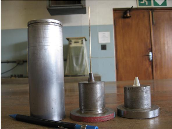
Figure 5.2 Mould for preparing specimens
