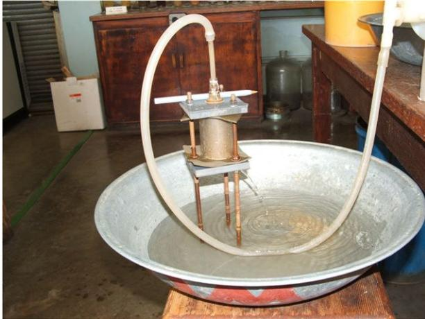
Figure 5.4 Set-up of the pinhole test
