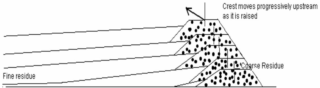
Figure 3.3 Upstream tailings dam construction (Klohn, 1980 and Blight, 1996).
