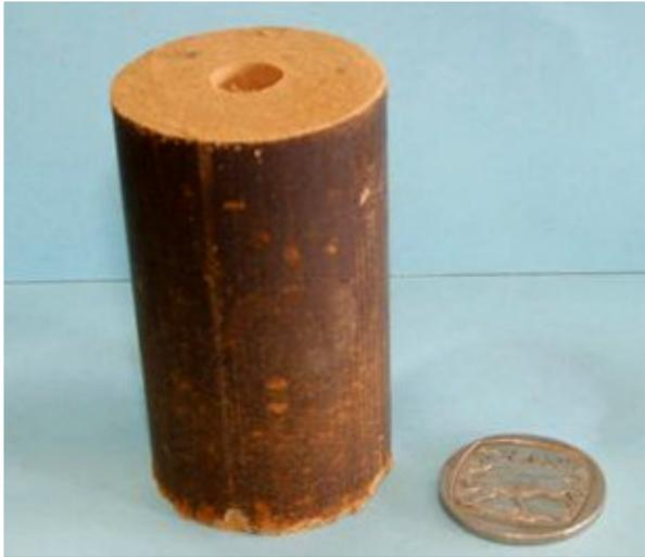
Figure 5.3 Pinhole specimens for gold tailing
