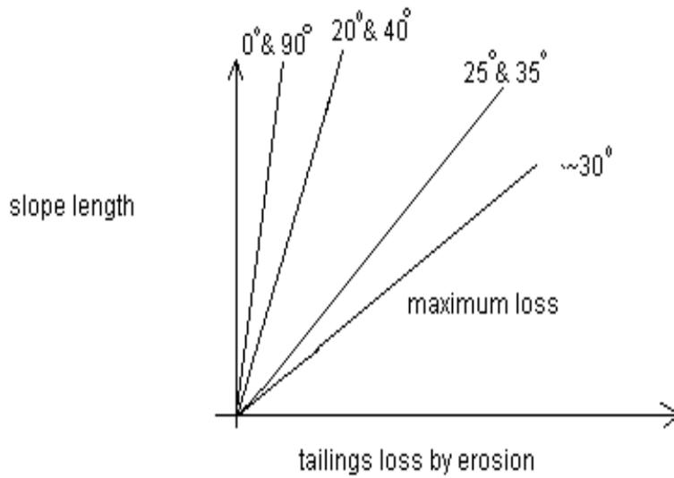
Figure 3.1 Effect of slope length on erosion of the outer slopes of tailings dams (Blight, 1996).
