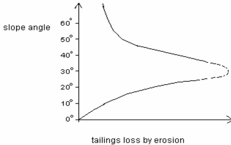
Figure 3.2 Effect of slope angle on erosion of the outer slopes of tailings dams (Blight, 1996).
