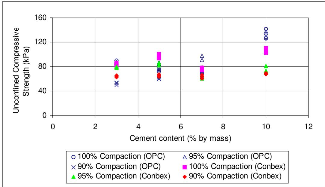
Figure 6.9 UCS for non-cured cement stabilized kimberlite (C2) tailings
