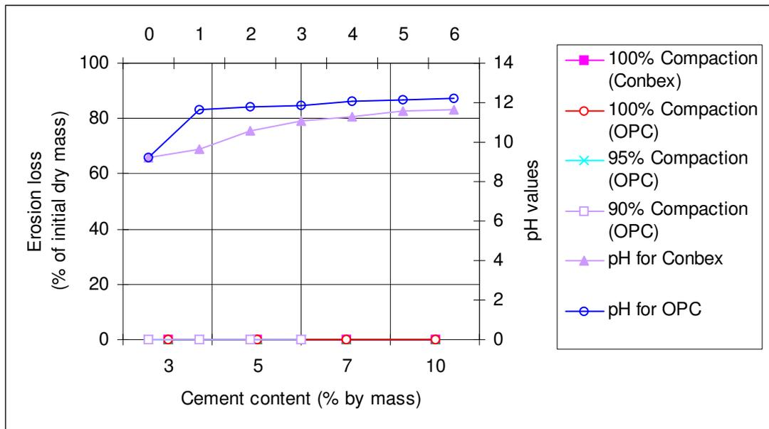
Figure 5.9 Analyses of the pinhole test for 7-days cured Kimberlite (C2) tailings
