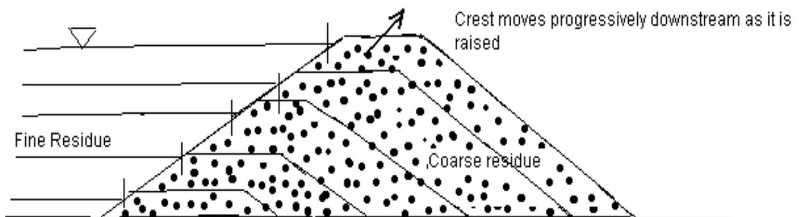
Figure 3.4 Downstream tailings dam construction (Klohn, 1980 and Blight, 1996).
