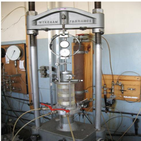
Figure 6.1 Apparatus for testing UCS
