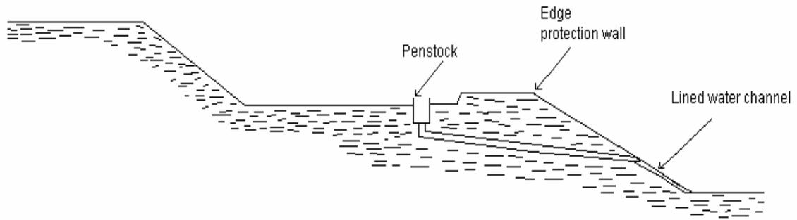
Figure 3.9 Erosion catchments berms (Chamber of Mines, 1996)
