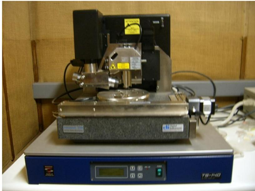
**Figure 4.13** The Dimension 3100 AFM/MFM apparatus on a vibration isolation table.
