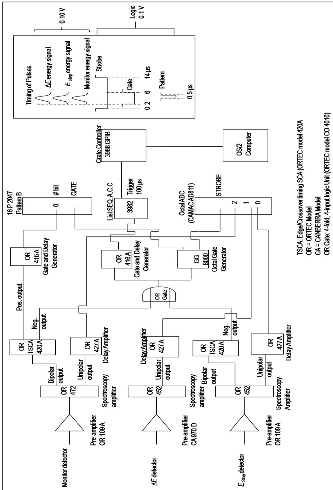
Figure 3.4: Block diagram of the data acquisition system.
