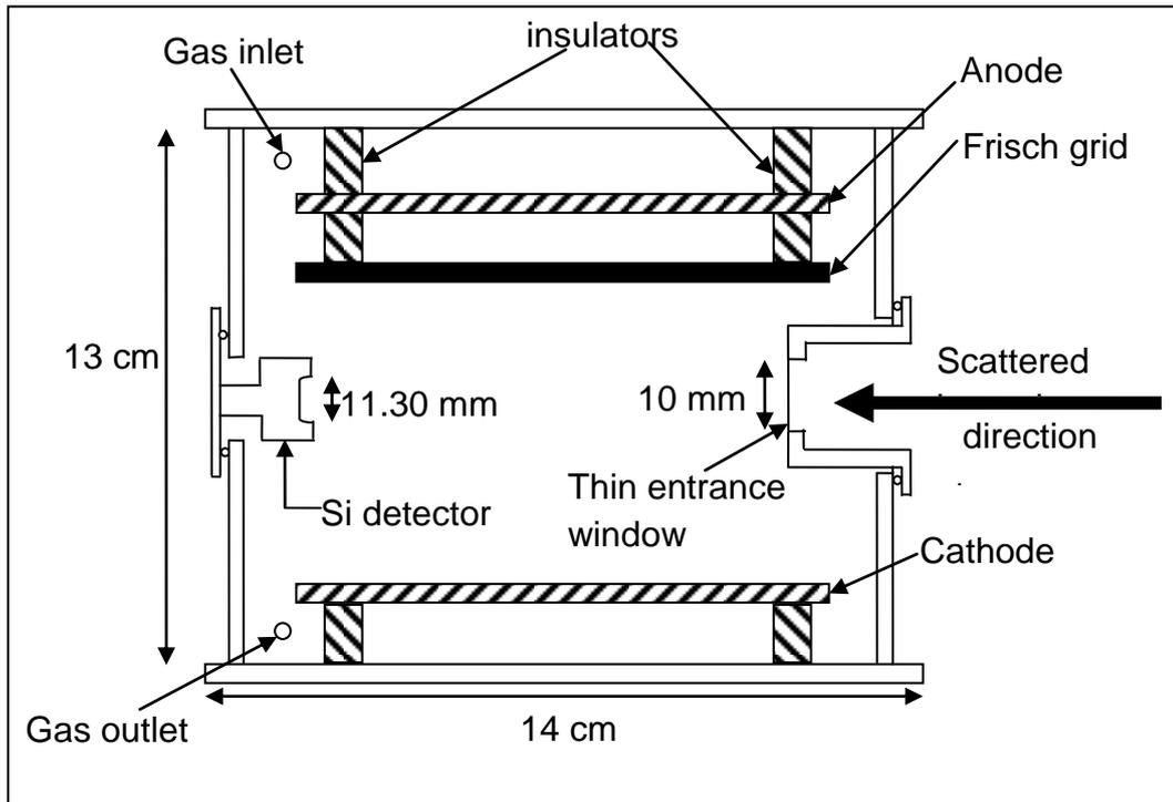
**Figure 3.3:**  $\Delta E$ - $E$  gas-ionisation detector.
