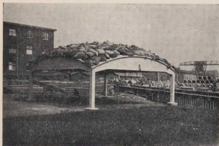
Fig. 8. Model of "surface of revolution" shell over 21ft. 6ins. bay, with shell thickness of 0.6in., being subjected to a test load of 16\frac{1}{2} tons.
