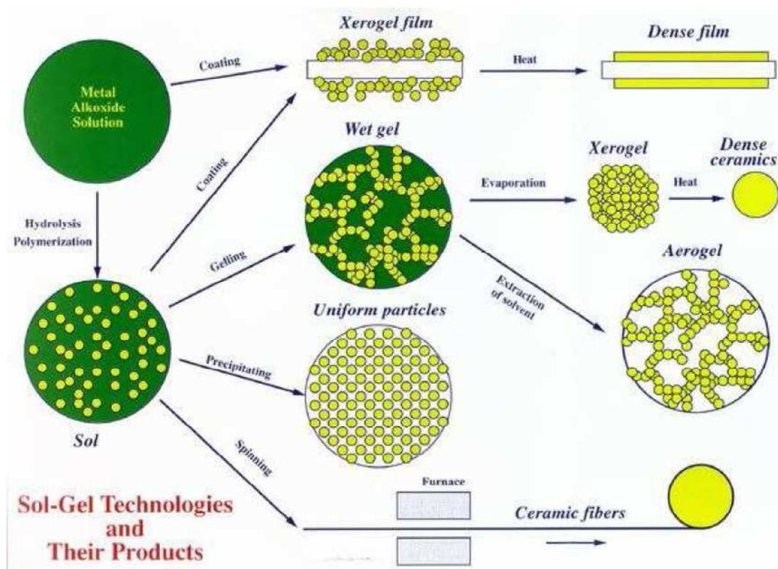
Figure 1.1 The sol-gel process and the various products formed.
