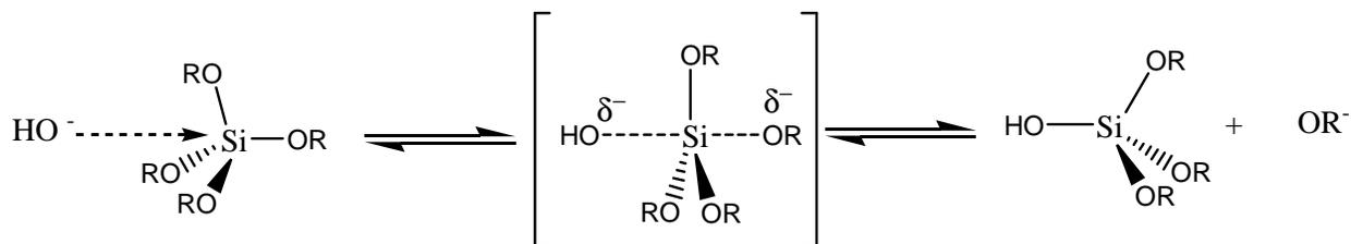
Scheme 1.2. Hydrolysis mechanisms of tetraalkylorthosilicate (R = alkyl).
