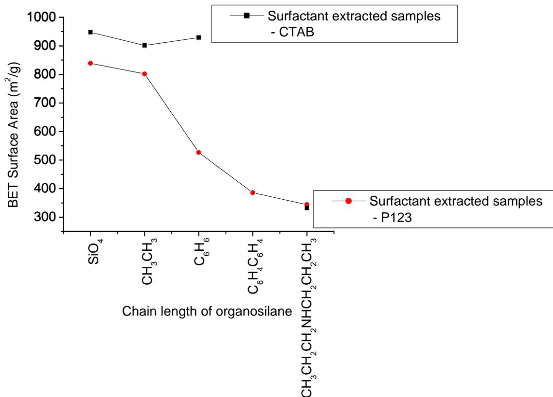
Figure 4.17 Graph showing the correlation between BET surface and the chain length of the organosilane.
