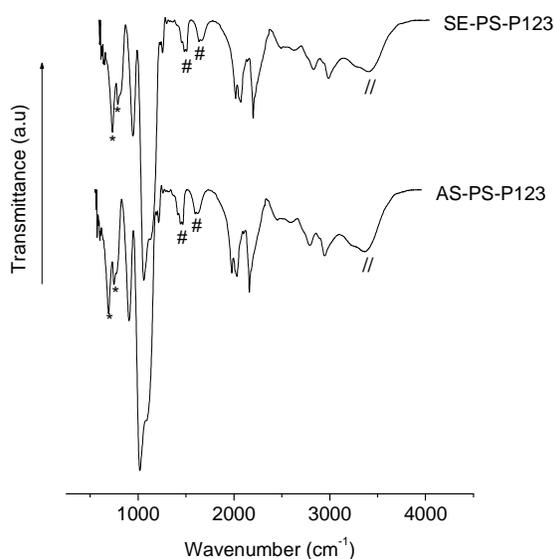
Figure 4.3 FTIR spectra of AS-PS-P123 and SE-PS-P123 mesoporous silica materials. (\*) modes assigned to Si – C stretching vibrations, (#) modes assigned to C – H stretching and deformation vibrations of Pluronic P123 and (//) modes assigned to N – H vibrations of the framework organic groups.
