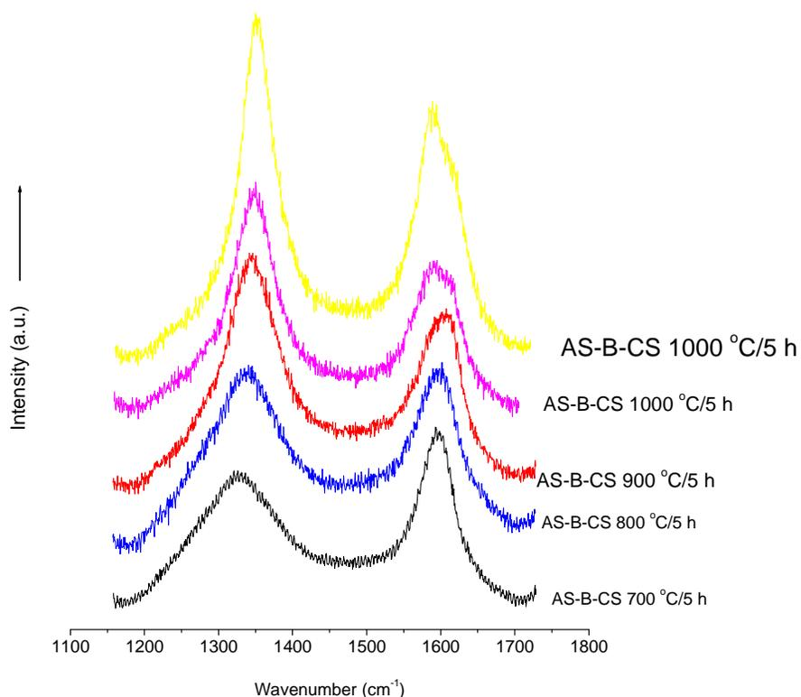
Figure 4.25 Raman spectra of a) AS-B-CS 700 °C/5 h, b) AS-B-CS 800 °C/5 h, c) AS-B-CS 900 °C/5 h, d) AS-B-CS 1000 °C/5 h and e) AS- B-CS 1100 °C/5 h carbon on silica nanocomposites samples.
