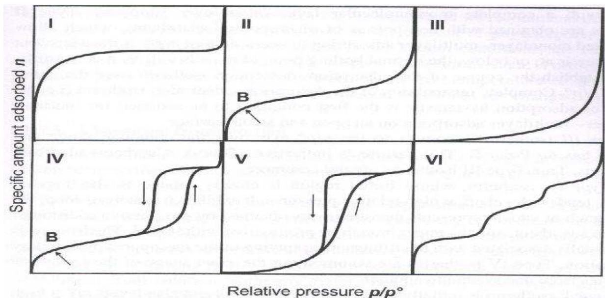
Figure 2.1 IUPAC classification of gas adsorption isotherms
