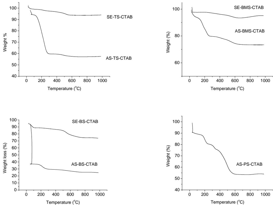
Figure 4.12 TGA curves of a) AS-TS-CTAB and SE-TS-CTAB, b) AS-BMS-CTAB and SE-BMS-CTAB, c) AS-BS-CTAB and SE-BS-CTAB, d) AS-PS-CTAB mesoporous silica materials.
