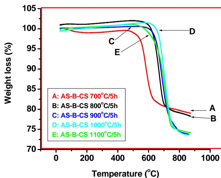
Figure 4.26 TGA curves of a) AS-B-CS 700 °C/5 h, b) AS-B-CS 800 °C/5 h, c) AS-B-CS 900 °C/5 h, d) AS-B-CS 1000 °C/5 h and e) AS-B-CS 1100 °C/5 h carbon on silica nanocomposites samples.
