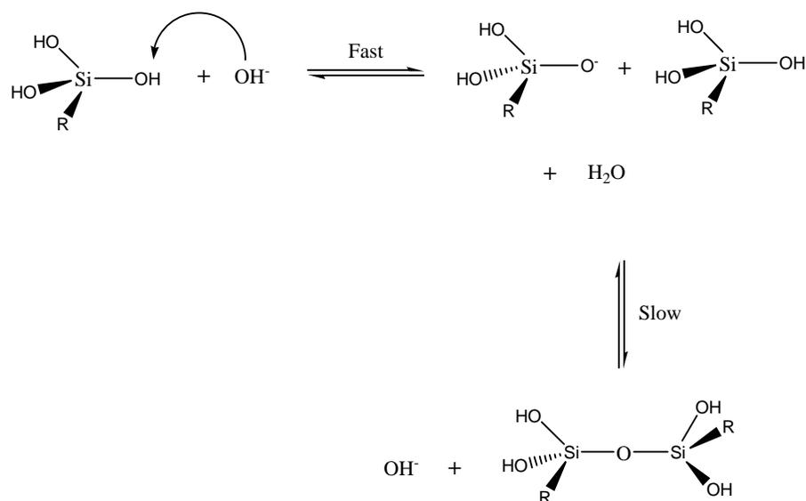
Scheme 1.3. Condensation mechanisms of tetraalkylorthosilicate (R = alkyl).
