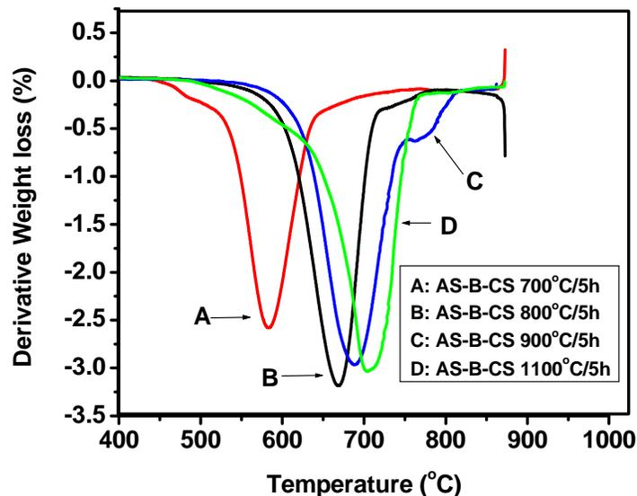
Figure 4.27 Derivative TGA curves of a) AS-B-CS 700 °C/5 h, b) AS-B-CS 800 °C/5 h, c) AS-B-CS 900 °C/5 h and d) AS-B-CS 1100 °C/5 h carbon on silica nanocomposite samples.
