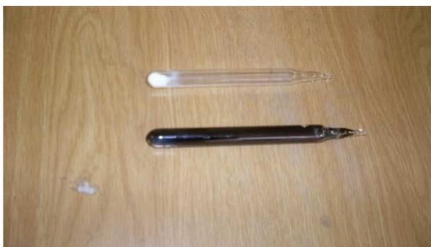
Figure 3.2: Pictures showing samples in quartz tubes, white sample before and black sample after the carbonization process.
