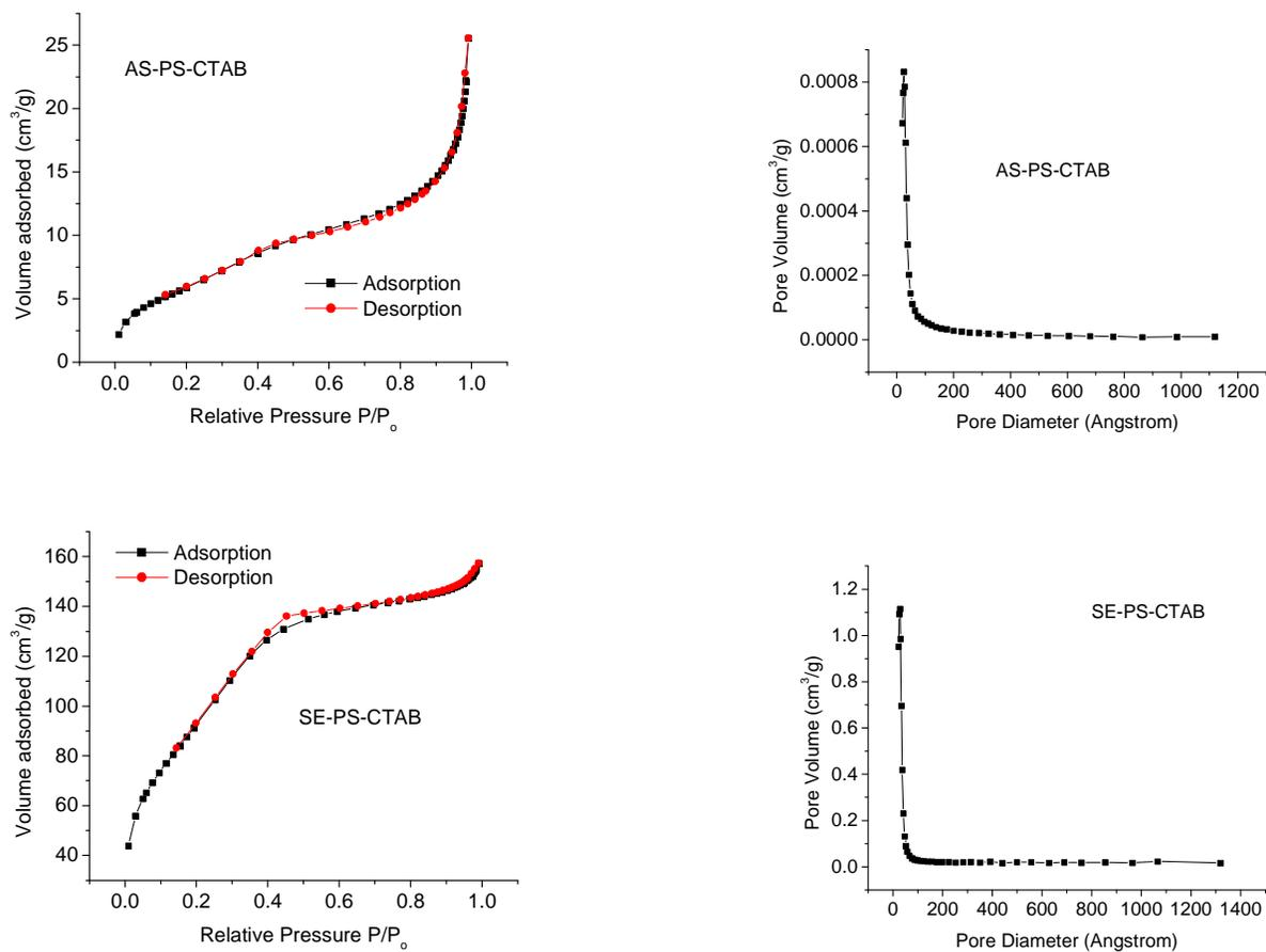
Figure 4.16 Nitrogen adsorption isotherms and the corresponding BJH pore size distributions derived from adsorption and desorption isotherms for a) AS-PS-CTAB and b) SE-PS-CTAB organosilica materials.
