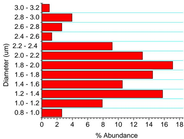
Figure 4.28 TEM images of AS-P-CS 1000 °C/0.5 h and the corresponding diameter distribution graph of carbon on silica beads.
