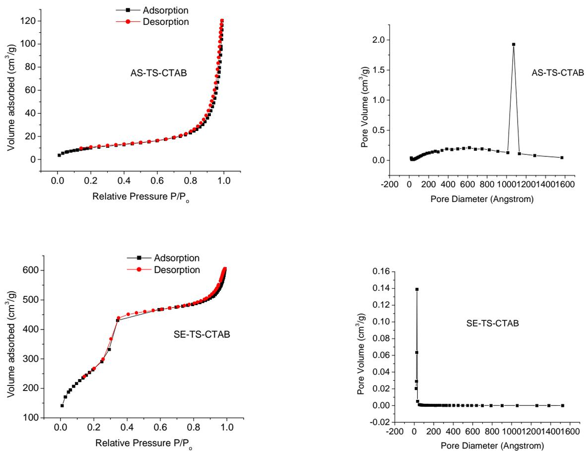
Figure 4.13 Nitrogen adsorption isotherms and the corresponding BJH pore size distributions derived from adsorption and desorption isotherms for a) AS-TS-CTAB and b) SE-TS-CTAB organosilica materials.
