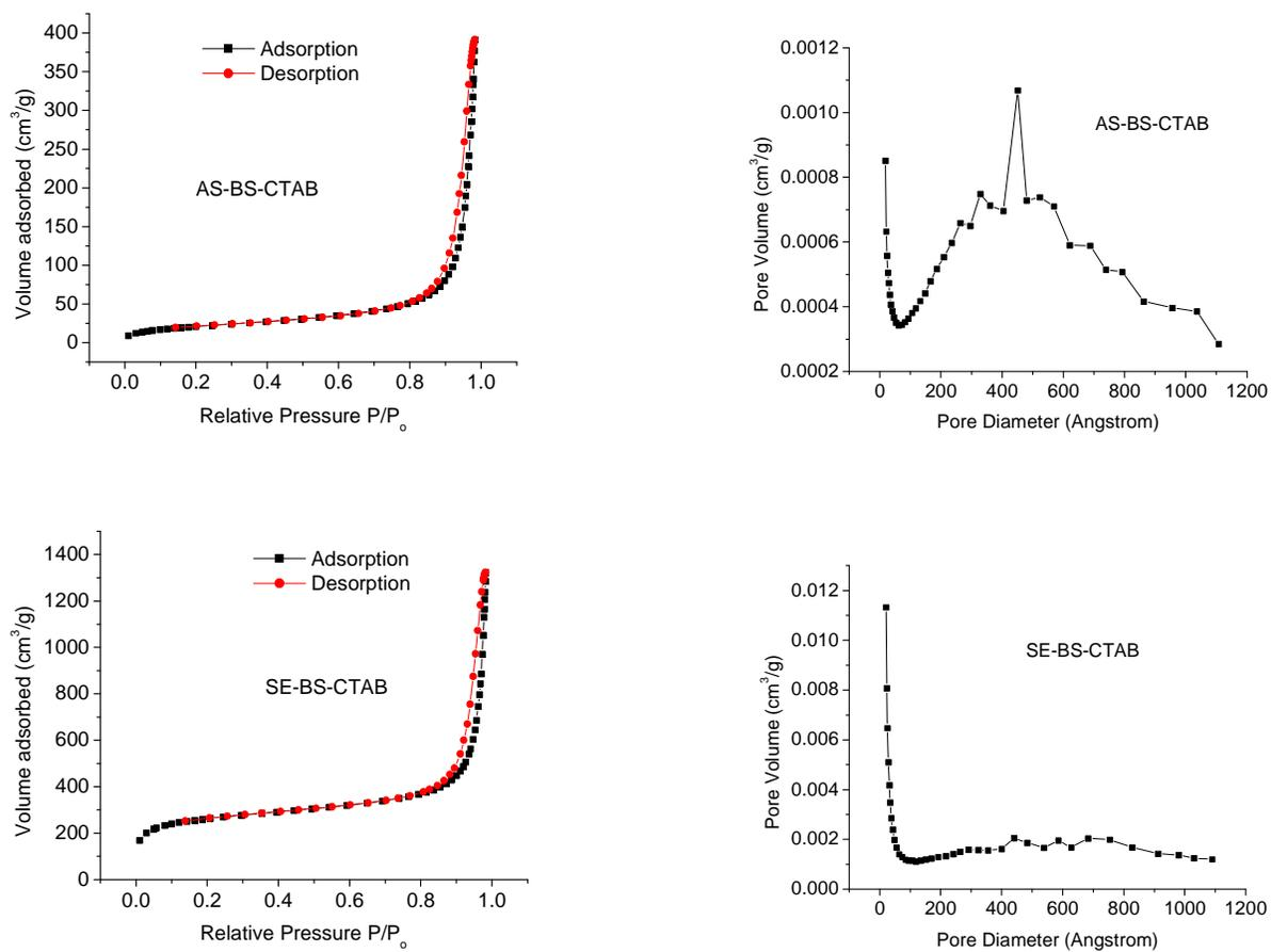
Figure 4.15 Nitrogen adsorption isotherms and the corresponding BJH pore size distributions derived from adsorption and desorption isotherms for a) AS-BS-CTAB and b) SE-BS-CTAB organosilica materials.
