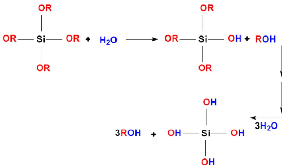
Scheme 1.1. Schematic representation of hydrolysis of tetraalkylorthosilicate (R = alkyl).
