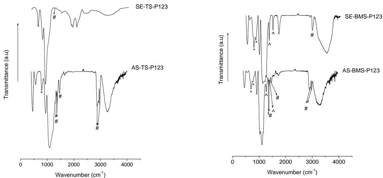
Figure 4.1 FTIR spectra of a) AS-TS-P123 and SE-TS-P123, b) AS-BMS-P123 and SE-BMS-P123 mesoporous silica materials. (\*) modes assigned to Si – C stretching vibrations, (#) modes assigned to C – H stretching and deformation vibrations of Pluronic P123 and (^) modes assigned to C – H deformation vibrations of the ethane framework organic groups.
