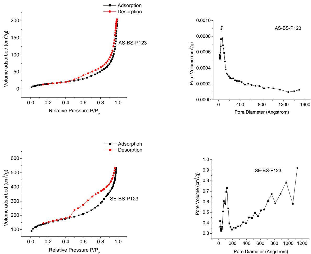
Figure 4.7 Nitrogen adsorption isotherms and the corresponding BJH pore size distributions derived from adsorption and desorption isotherms for a) AS-BS-P123 and b) SE-BS-P123 organosilica materials.
