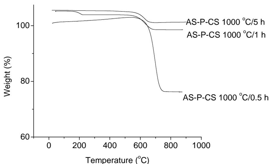
Figure 4.31 TGA curves of a) AS-P-CS 1000 °C/5 h, b) AS-P-CS 1000 °C/1 h and c) AS-P-CS 1000 °C/0.5 h carbon on silica nanocomposites samples.
