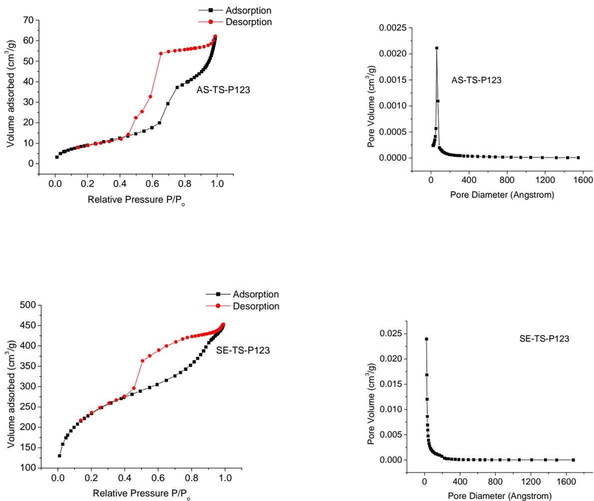
Figure 4.5 Nitrogen adsorption isotherms and the corresponding BJH pore size distribution curves derived from adsorption and desorption isotherms for a) AS-TS-P123 and b) SE-TS-P123 organosilica materials.
