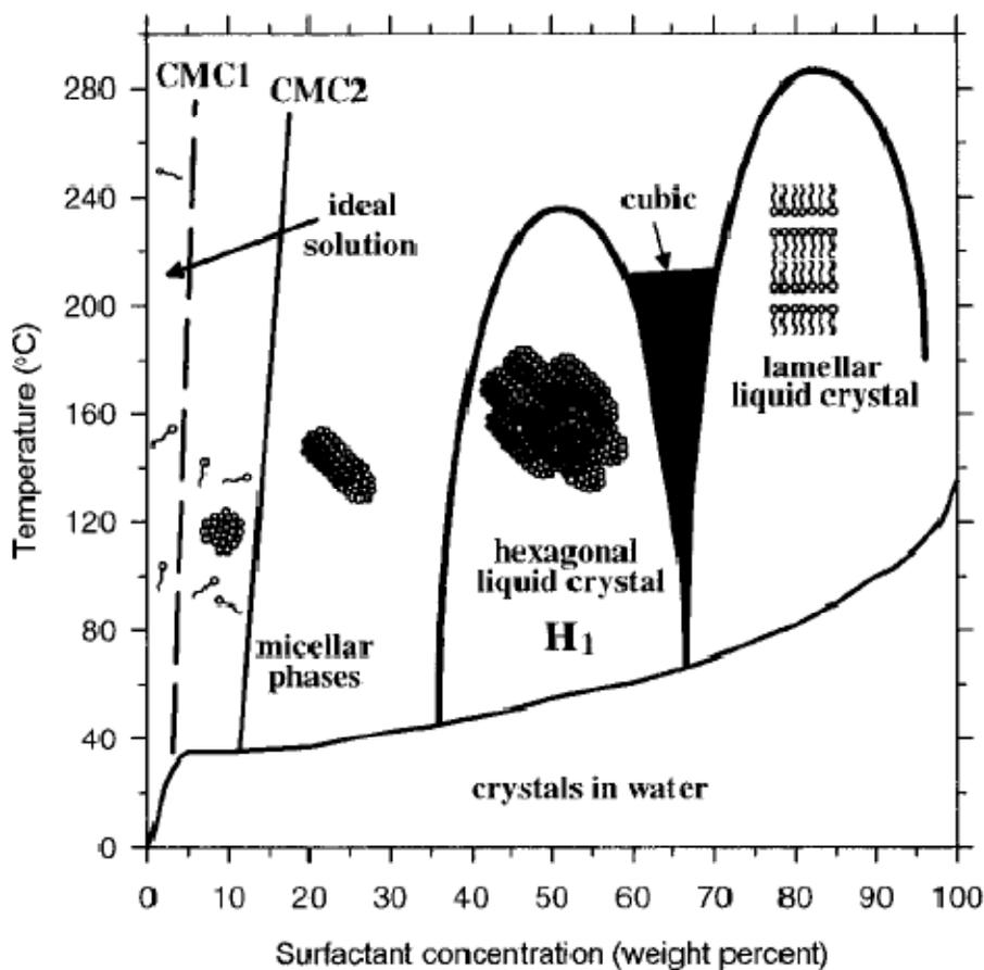
Figure 1.3. Schematic phase diagram for CTAB in water.
