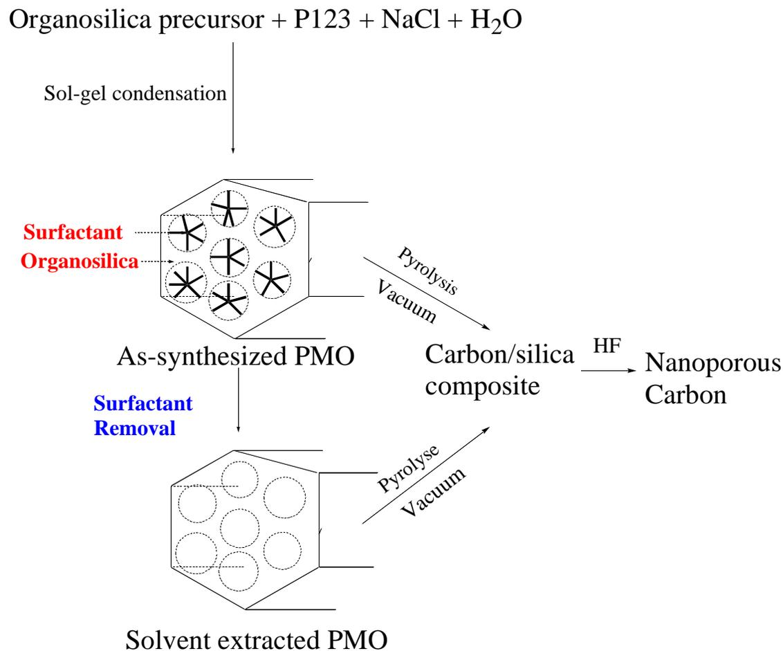
Figure 3.1 Schematic showing the formation of as-synthesized and extracted periodic mesoporous organo-bridged silica, carbon/silica composites and mesoporous carbons.
