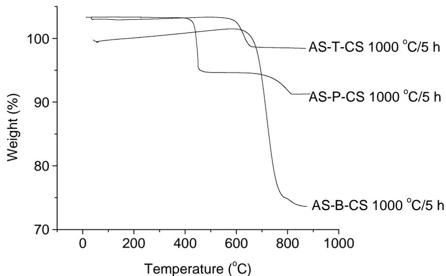
Figure 4.23 TGA curves of a) AS-T-CS 1000 °C/5 h, b) AS-P-CS 1000 °C/5 h and c) AS-B-CS 1000 °C/5 h samples.
