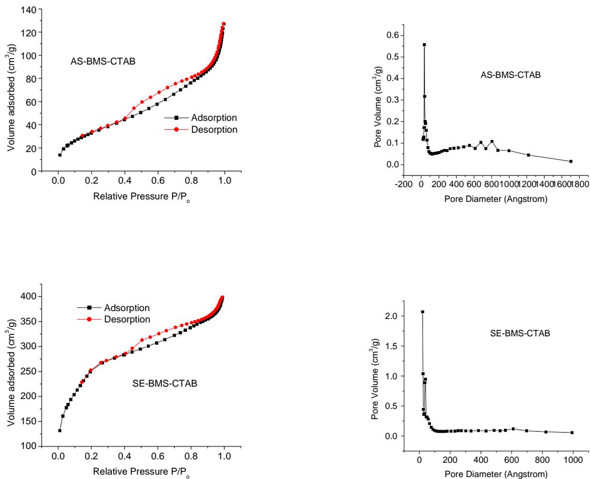
Figure 4.14 Nitrogen adsorption isotherms and the corresponding BJH pore size distributions derived from adsorption and desorption isotherms for a) AS-BMS-CTAB and b) SE-BMS-CTAB organosilica materials.
