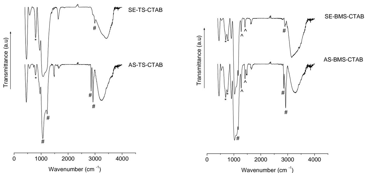
Figure 4.10 FTIR spectra of a) AS-TS-CTAB and SE-TS-CTAB and b) AS-BMS-CTAB and SE-BMS-CTAB mesoporous silica materials. (\*) modes assigned to Si – C stretching vibrations, (#) modes assigned to C – H stretching and deformation vibrations of CTAB and (^) modes assigned to C – H deformations vibrations of the framework organic group.
