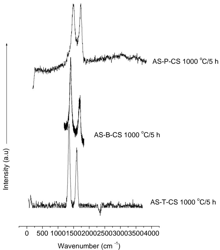
Figure 4.22 Raman spectra of a) AS-T-CS 1000 °C/5 h, b) AS-B-CS 1000 °C/5 h and c) AS-P-CS 1000 °C/5 h samples.
