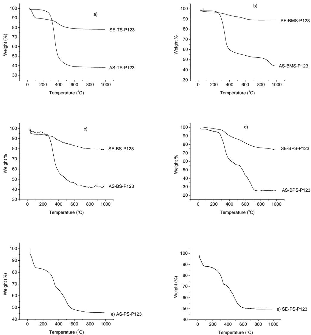
Figure 4.4 TGA curves of a) AS-TS-P123 and SE-TS-P123, b) AS-BMS-P123 and SE-BMS-P123, c) AS-BS-P123 and SE-BS-P123, d) AS-BPS-P123 and SE-BPS-P123 and e) AS-PS-P123 mesoporous silica materials.
