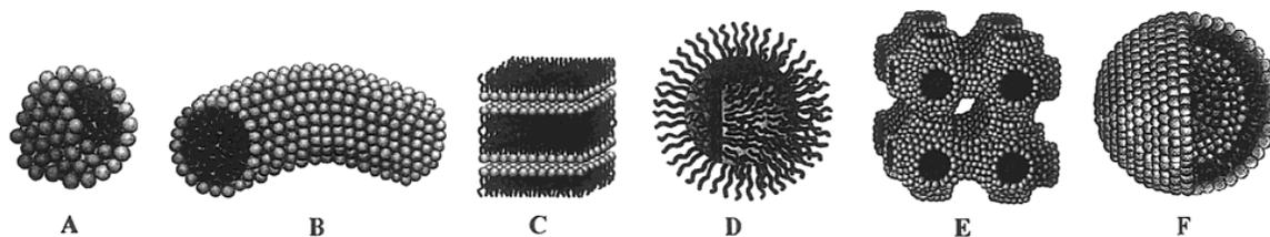
Figure 1.2 Supramolecular structures for surfactants. (A = sphere, B = cylinder, C = planar bilayer, D = reverse micelle, E = bicontinuous phase and F = liposomes).
