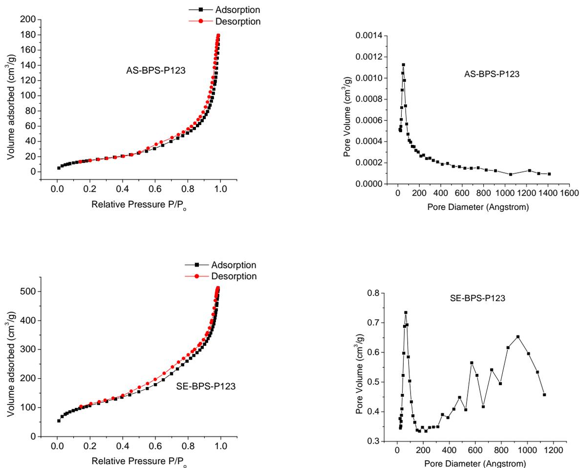
Figure 4.8 Nitrogen adsorption isotherms and the corresponding BJH pore size distributions derived from adsorption and desorption isotherms for a) AS-BPS-P123 and b) SE-BPS-P123 organosilica materials.
