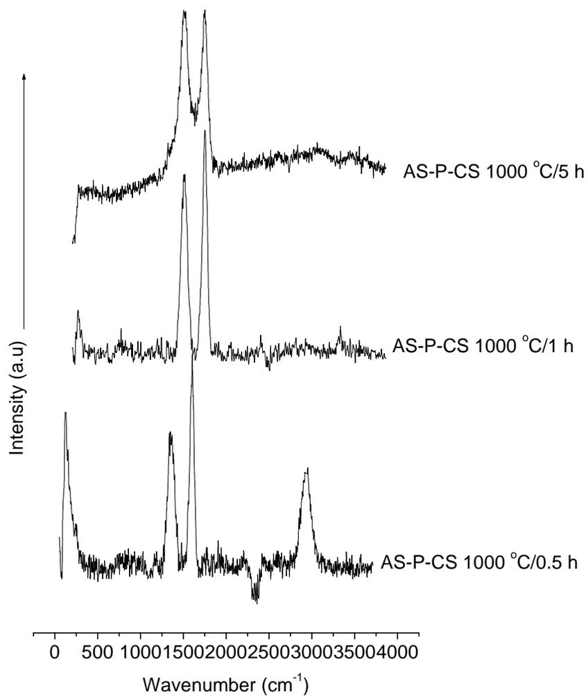
Figure 4.32 Raman spectra of a) AS-P-CS 1000 °C/5 h, b) AS-P-CS 1000 °C/1 h and c) AS-P-CS 1000 °C/0.5 h carbon on silica nanocomposite samples.
