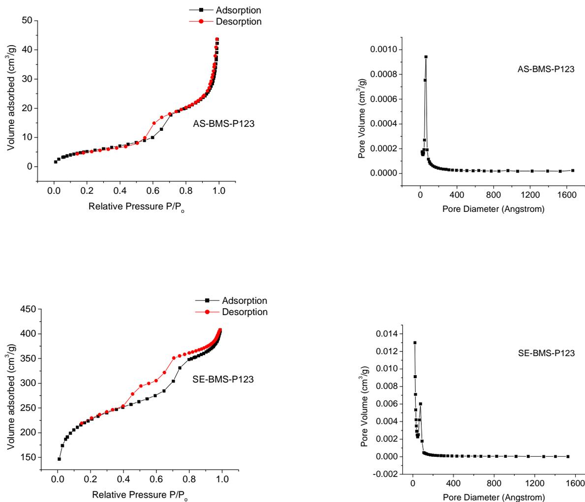
Figure 4.6 Nitrogen adsorption isotherms and the corresponding BJH pore size distributions derived from adsorption and desorption isotherms for a) AS-BMS-P123 and b) SE-BMS-P123 organosilica materials.
