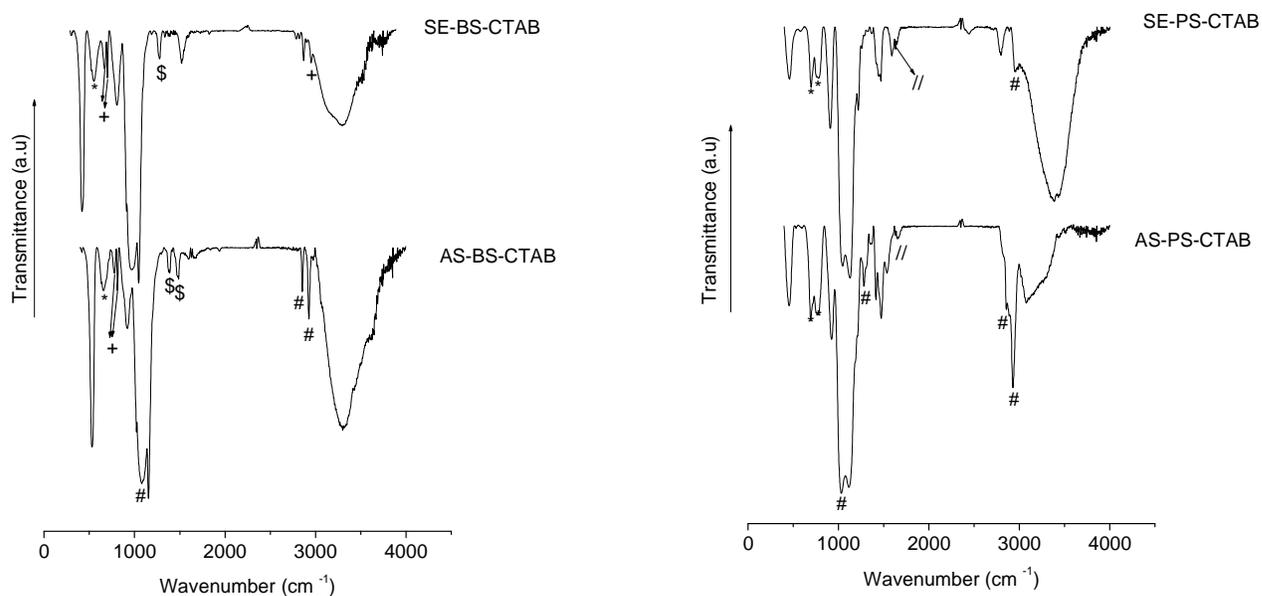
Figure 4.11 FTIR spectra of a) AS-BS-CTAB and SE-BS-CTAB and b) AS-PS-CTAB and SE-PS-CTAB mesoporous silica materials. (\*) modes assigned to Si – C stretching vibrations, (#) modes assigned to C – H stretching and deformation vibrations of CTAB, (\$) modes assigned to C – C stretching vibrations of the aromatic ring, (+) modes assigned to C – H stretching vibrations of the aromatic ring and (//) modes assigned to N – H bend vibrations.
