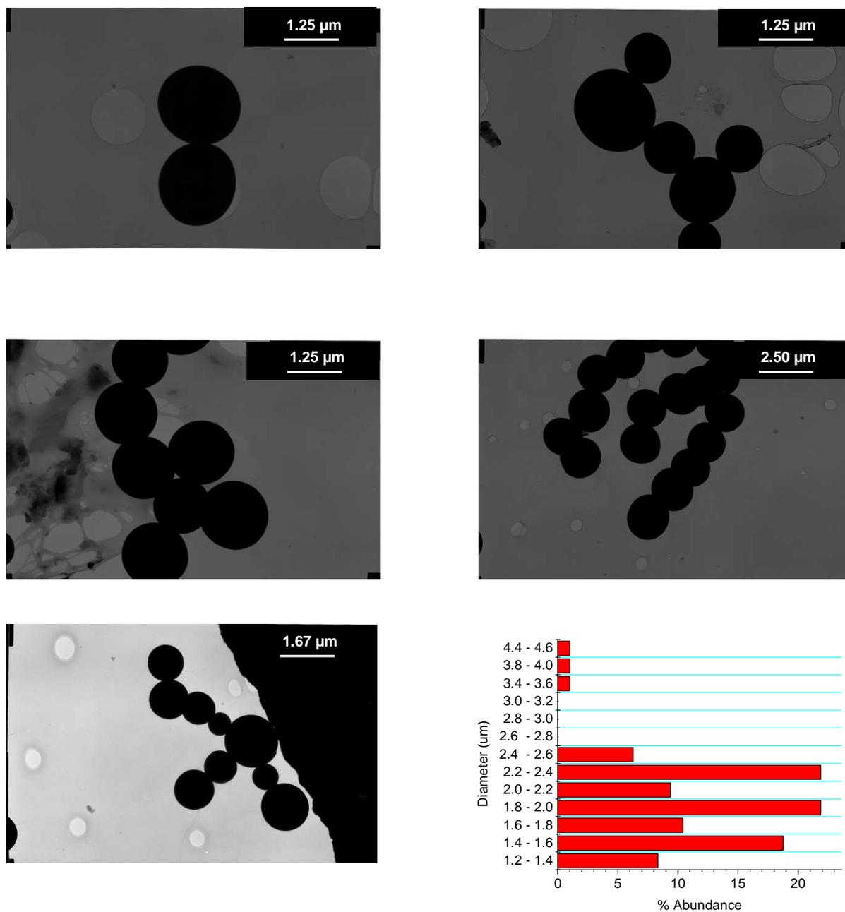
Figure 4.29 TEM images of AS-P-CS 1000  $^{\circ}\text{C}/1\text{ h}$  and the corresponding diameter distribution graph of carbon on silica beads.
