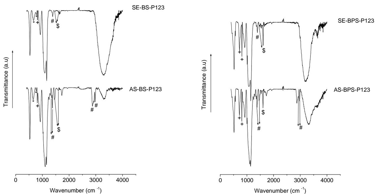
Figure 4.2 FTIR spectra of a) AS-BS-P123 and SE-BS-P123, b) AS-BPS-P123 and SE-BPS-P123 mesoporous silica materials. . (\*) modes assigned to Si – C stretching vibrations, (#) modes assigned to C – H stretching and deformation vibrations of Pluronic P123, (\$) modes assigned to C – C stretching vibrations of the aromatic ring and (+) modes assigned to C – H absorption bands of the aromatic ring.
