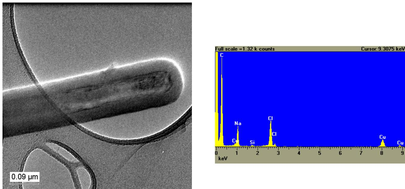
Figure 4.21 High magnification TEM images and corresponding EDX spectra of AS-P-CS 1000 °C/5 h carbon on silica nanocomposite sample.
