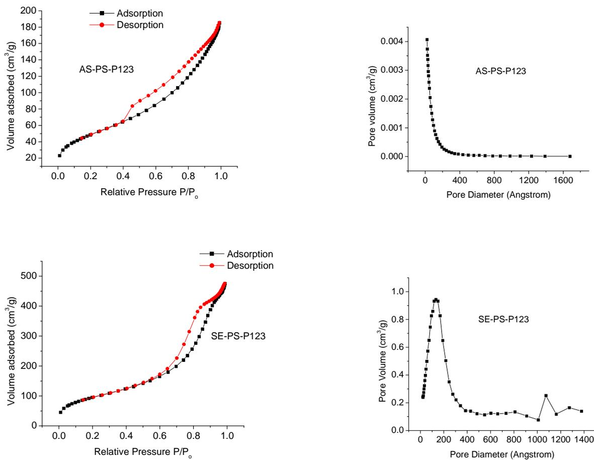
Figure 4.9 Nitrogen adsorption isotherms and the corresponding BJH pore size distributions derived from adsorption and desorption isotherms for a) AS-PS-P123 and b) SE-PS-P123 organosilica materials.
