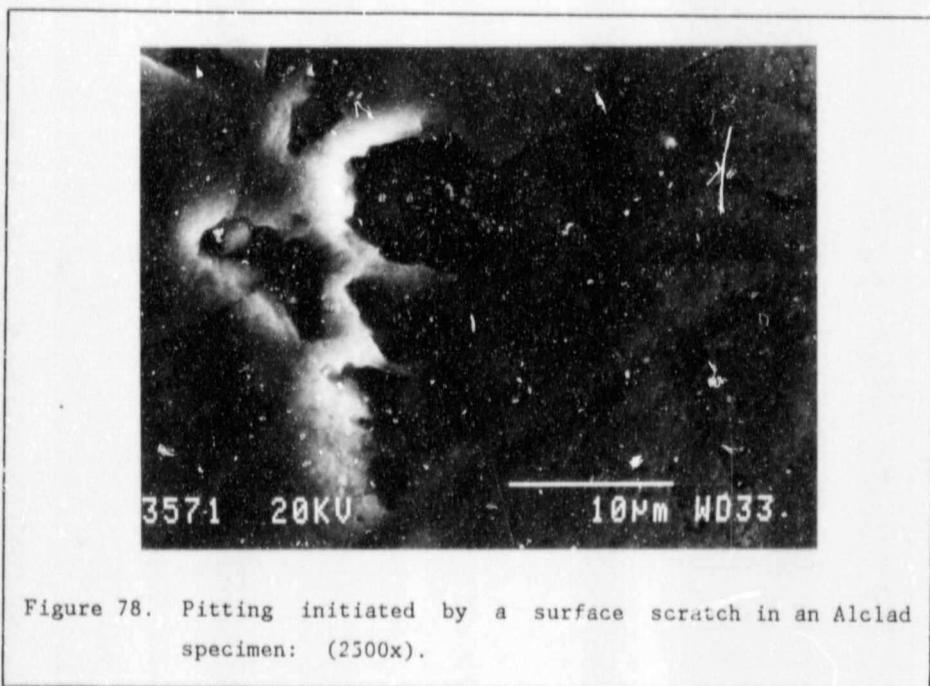
Figure 78. Pitting initiated by a surface scratch in an Alclad specimen: (2500x).
